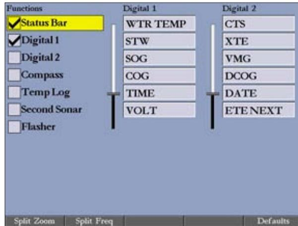
2. Using the **ROCKER**, highlight the function you want to add or remove, and press **ENTER**. Only functions with a check mark in the check box next to them appear on the Sonar Page.
