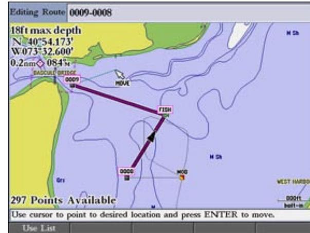
4. Use the **ROCKER** to drag the map pointer to the location where you want to move the route point, and then press **ENTER** to move the route point.
