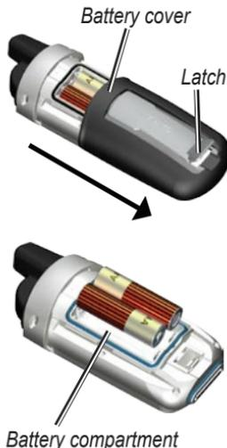
**NOTE:** Remove batteries when you do not plan to use the Colorado for several months. Stored data is not lost when batteries are removed.
