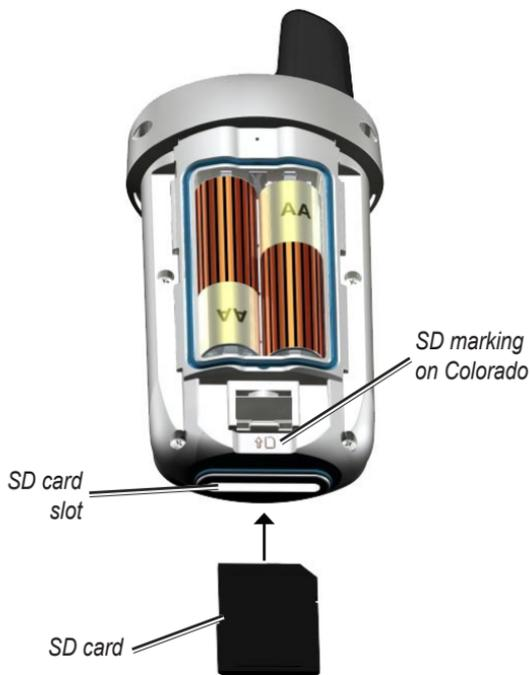
**Inserting an SD Card into the Colorado**
