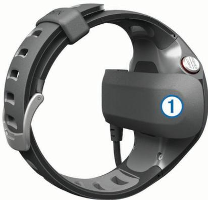
When you connect the device to a power source, the device turns on, and the charging screen appears.
