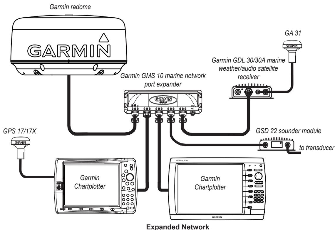
**NOTE:** When using the Garmin radome with an expanded network, each network component must be installed according to its installation instructions. This diagram only shows how a Garmin radome communicates with an expanded network, and does not show the full wiring needs of the other network components.
