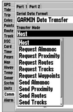
When transferring data between two Garmin units, always set one to Host and use the other unit to either Send or Request the data.
