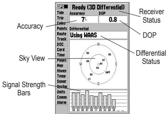
The status field indicates a 2D or 3D, when the GPSMAP 188/188C Sounder has collected the necessary data from satellites to calculate a fix. The unit then updates the location, date, and time.
