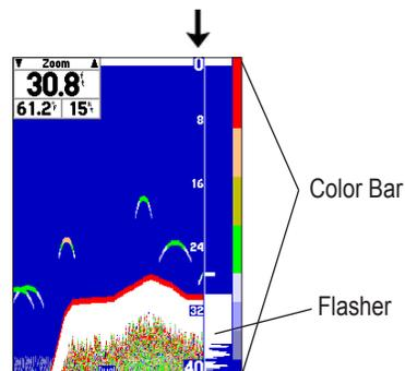
**Flasher**—with the Flasher active, a graphic Flasher representation is displayed on the far right side of the graph. This graphic Flasher displays structure and bottom returns much the same as a true Flasher. This feature is particularly useful when using fish symbols.
