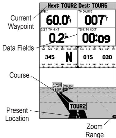
You can zoom in or out on the Highway display for a smaller or larger view. Five available settings range from 1X to 16X, with a default setting of 8X. The current range appears in the bottom right of the display.
