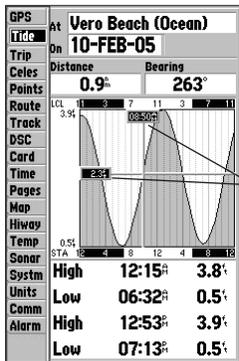
Move the pointer to see tide heights at different times. Tide data shows in a black box when in pointer mode.
