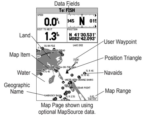
The GPSMAP 188/188C Sounder system starts in the Position Mode, with your location centered on the map display. When sufficient map coverage is not available to keep your location centered, the position triangle moves toward the edge of the display.
