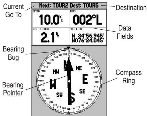
The Pointer Page features a menu page that provides access to layout and data field options. The data window, located at the top of the page, provides a user-selectable layout of various types of useful data. Each data field can be configured to display several data options. The data window layout can be configured to display additional data fields and change the size of the data displayed.
