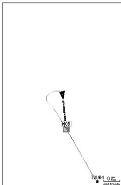
The MOB function allows you to quickly activate navigation back to a location.
