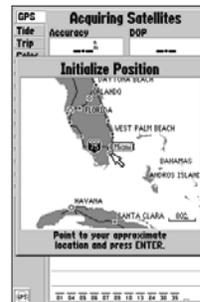
The unit now begins searching for the appropriate satellites for your region and should acquire a fix within a few minutes. When viewing the GPS tab on the Main Menu, a signal strength bar for each satellite in view appears on the bottom of the page, with the appropriate satellite number under each bar.
