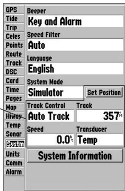
The Set Position, Track Control, Track and Speed fields only show while in Simulator Mode.
