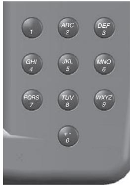
Use the shortcut keys to jump to main pages, or select menu and list options by pressing the corresponding number of the selection. For numbers 1-9, press the number to choose the selection. For numbers 10 and higher, press the first digit, then press the second digit within one second.
