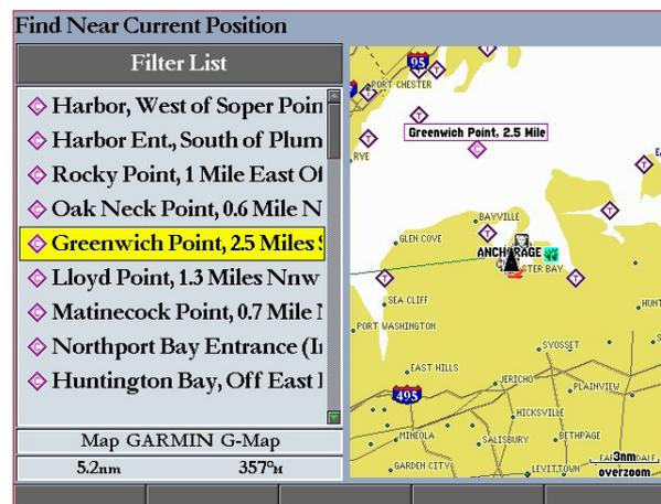
3. Select a Current Station from the list, and press **ENTER**. As you move the highlight over each Current Station in the list, the station is highlighted on the map window. The distance and bearing from your location to the highlighted station are shown at the bottom of the list.
