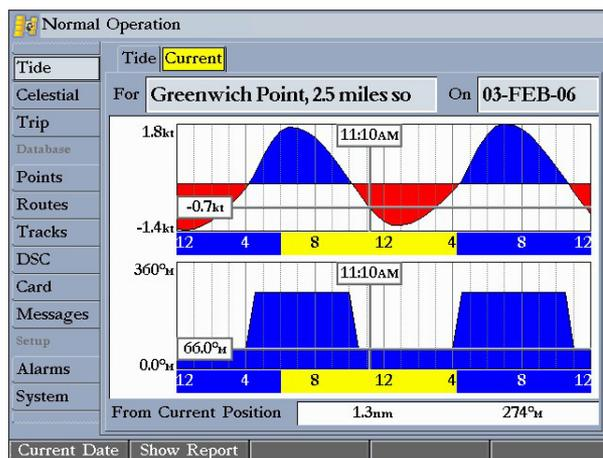
The Current sub tab contains two charts, one for speed and one for direction.
