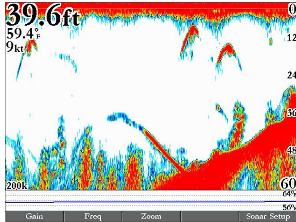
The sonar function window contains a right-to-left moving sonar image of the water beneath your boat. Items appear as they pass under the transducer. The most recent data is shown on the right side of the screen. The right side of the screen contains a scale reflecting the depth of the area being shown. The top-left corner shows the depth, water temperature, and speed through water (if equipped with a temperature or speed sensor).
