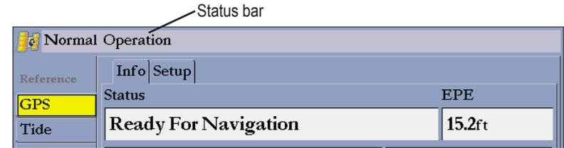
Alarm alerts also appear on the status bar. To acknowledge an alarm, press **QUIT**. If an alarm condition persists, it appears on the status bar until the alarm condition no longer exists. For more information about alarms, see pages [56-58](#).
