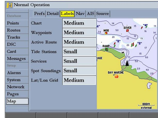
**Chart**, **Waypoints**, **Active Route**, **Tide Stations**, **Services**, **Spot Soundings**, **Lat/Lon Grid**—controls the screen size of the text for a given map item. Select **None**, **Small**, **Medium**, or **Large**.
