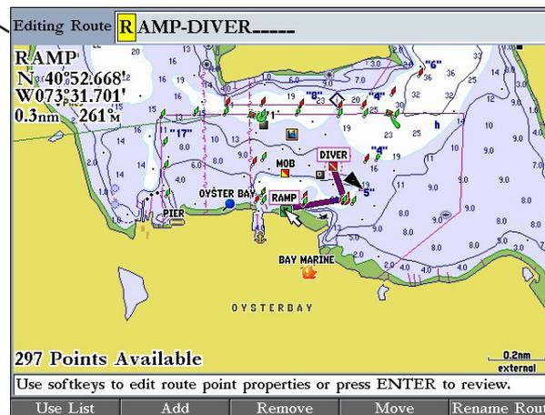
3. Use the **ROCKER** or data entry keys to change the route name, and press **ENTER** when finished.
