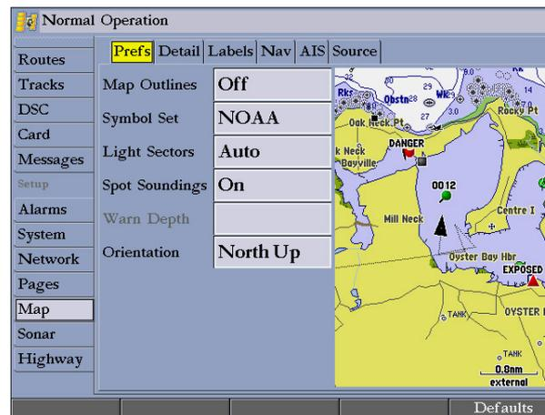
2. Press left or right on the **ROCKER** to highlight a sub tab, press up or down to highlight the setting you want to change, and press **ENTER**.
