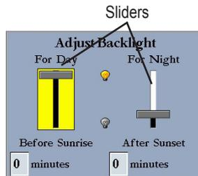
5. Press up or down on the **ROCKER** to increase or decrease the backlight level, and press **ENTER**.
