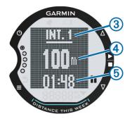
The paused screen includes the interval number ③, interval distance ④, and swim time for the interval ⑤. The screen appears inverted until you select II and resume swimming.
