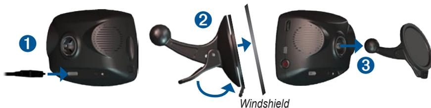
1. Plug the power cable into the power connector on the back of the c510.
