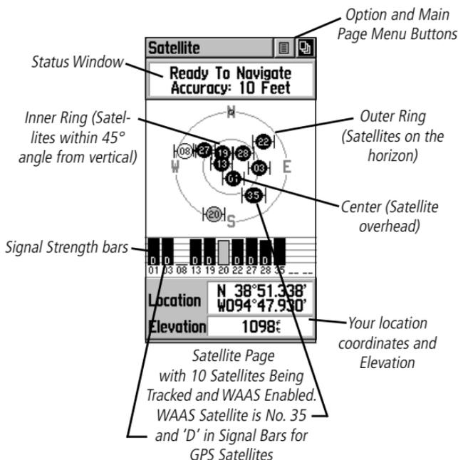
The Satellite Page provides a picture of satellite signal tracking, tells you when the unit is ready for navigation, and shows your location coordinates.
