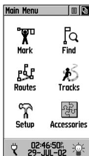
*The Main Menu Page with Feature Icons and Battery Capacity, Time/Date, and Backlighting Status Bar.*
