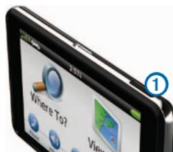
**NOTE:** If you hold the Power key for less than 4 seconds, the device enters sleep mode.
