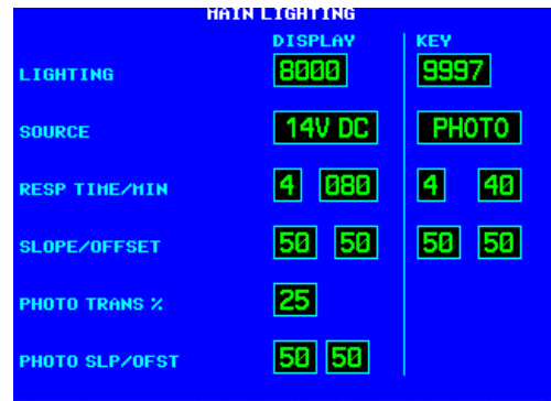
Figure 5-9. Main Lighting Page with Alternate Source
