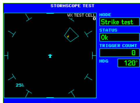
Figure 5-20. STORMSCOPE TEST Page
