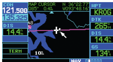
Figure 7-40 Activate Panning Function
