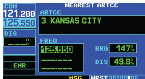
Figure 8-22 Frequency Moved to Standby Field
