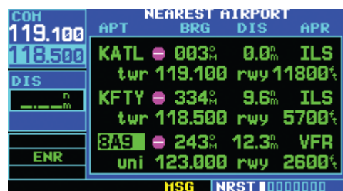
Figure 8-10 Frequency Moved to Standby Field
