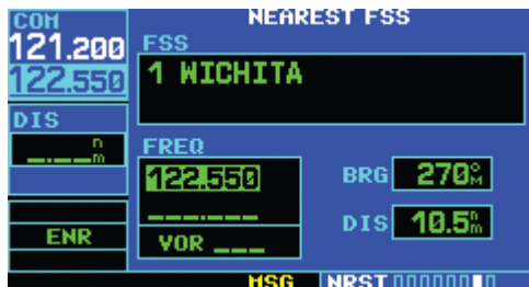
Figure 8-26 Frequency Moved to Standby Field
