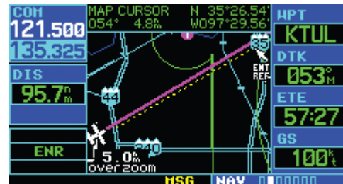
Figure 3-21 Using Pointer to Measure Distance and Bearing
