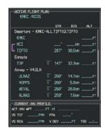
Figure 8-3 Active Flight Plan Page on the MFD
