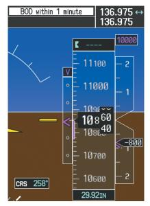
Figure 7-40 Approaching Bottom of Descent (BOD) at OPSHN
