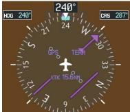
Figure 7-11 Assigned Heading of 240°
