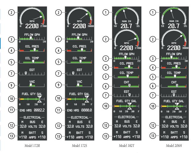
Figure 3-1 Engine Display (Normally-aspirated Aircraft)
