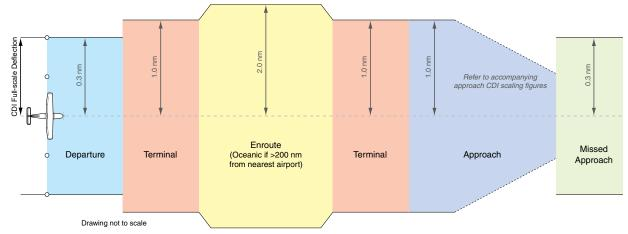
Figure 2-22 Phases of Flight/CDI Scaling
