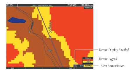
Figure 10-44 Navigation Map Page (After TERRAIN-SVS Pop-up Alert Acknowledgment)
