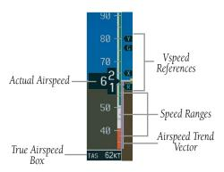
Figure 2-4 Airspeed Indicator
