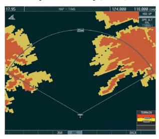
Figure 10-48 TAWS-B Page (ARC View)
