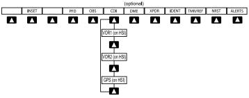
Figure 1-2 PFD Top Level Softkeys
