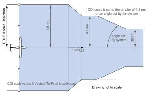
Figure 2-23 Typical LNAV and LNAV+V Approach CDI Scaling
