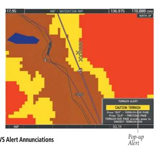
Figure 10-43 TERRAIN-SVS Alert Annunciations
