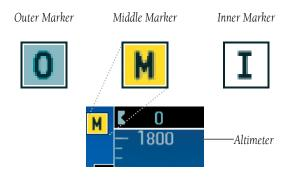
Figure 5-4 Marker Beacon Annunciators on the PFD
