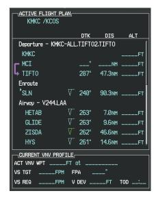
Figure 7-13 Begin Adding V4 to the Flight Plan
