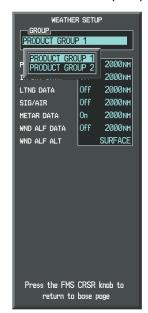
Figure 10-18 Weather Data Link (GFDS) Page Setup Menu
