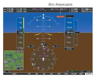
Figure 10-53 TAWS Alert Annunciation on the PFD
