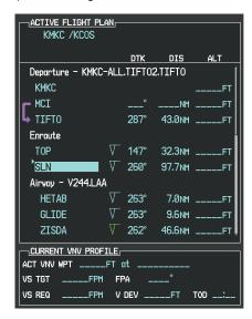
Figure 7-15 TOP Inserted into the Flight Plan
