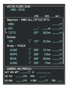
Figure 7-19 V4 is Loaded in the Flight Plan
