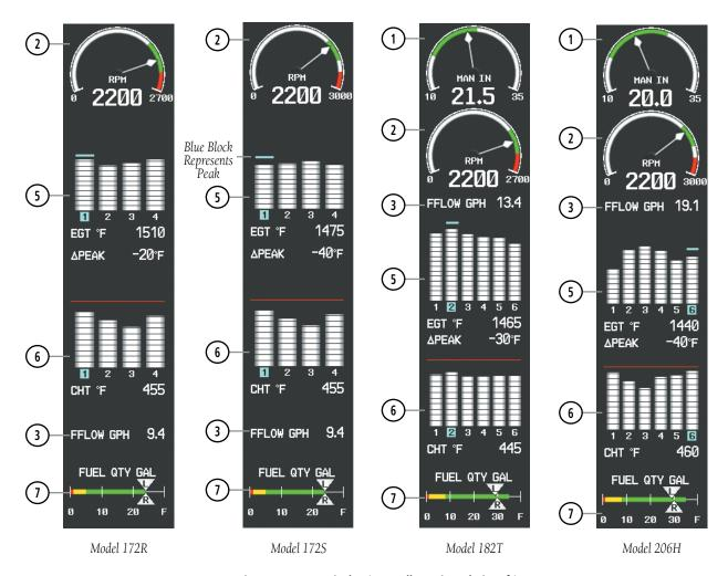
Figure 3-3 Lean Display (Normally-aspirated Aircraft)
