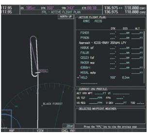
Figure 7-50 Establishing the Holding Pattern
