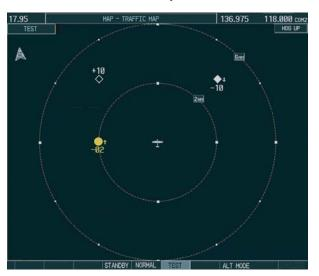
Figure 10-33 Self Test OK Display
