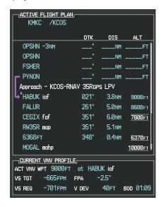
Figure 7-35 Vertical Guidance is Active to the FAF
