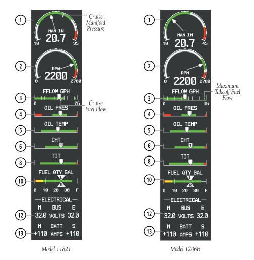
Figure 3-2 Engine Display (Turbocharged Aircraft)
