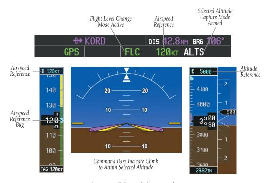
Figure 6-9 Flight Level Change Mode
