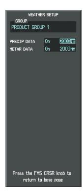
Figure 10-10 Weather Data Link Page Setup Menu
