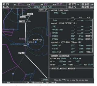
Figure 7-42 Tracking the OPSHN to FSHER Leg
