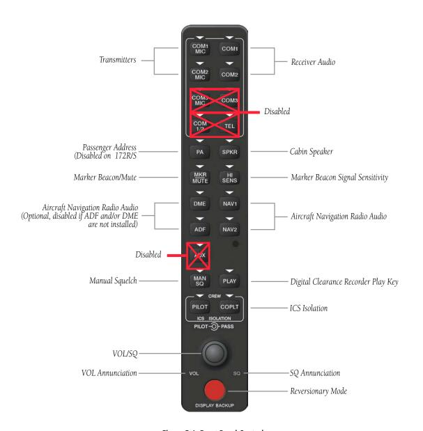
Figure 5-1 Front Panel Controls
