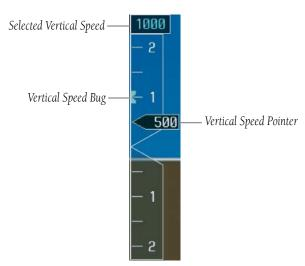
Figure 2-15 Vertical Speed Indicator
