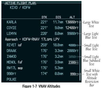
Some altitudes retrieved from the database have associated restrictions indicating to stay 'At', 'At or Above', or 'At or Below' a specific altitude. These restrictions are indicated using a 'bar' above and/or below the appropriate altitude as shown in Figure 1-9.
