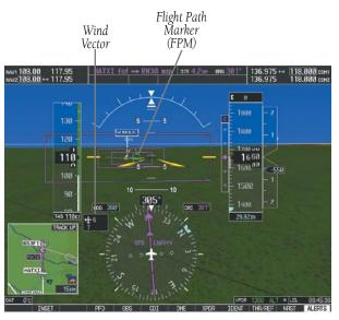
Figure 11-6 Flight Path Marker and Pathways
