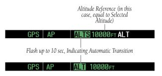
Figure 6-6 Automatic Mode Transitions During Altitude Capture
