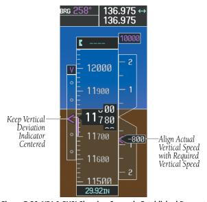
Figure 7-39 VDI & RVSI Showing Correctly Established Descent
