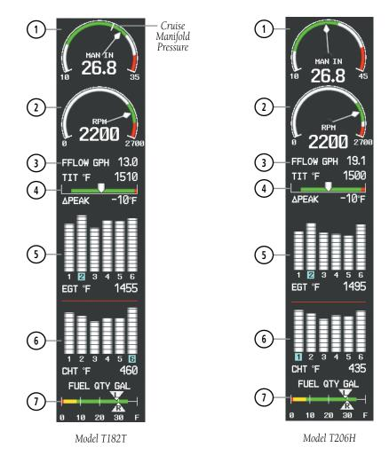
Figure 3-4 Lean Display (Turbocharged Aircraft)
