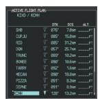
Figure 8-20 Airway Added to Flight Plan
