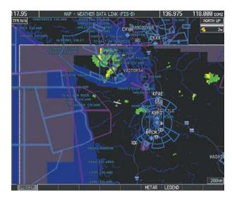
Figure 10-14 Weather Data Link Page(FIS-B) PRECIP
