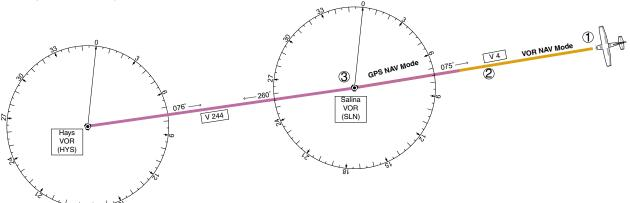
Figure 6-33 Transition to GPS Flight Plan
