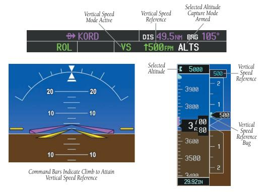
Figure 6-8 Vertical Speed Mode
