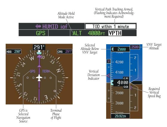
Figure 6-11 Vertical Path Capture
