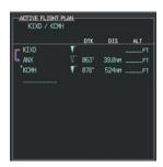
Figure 8-17 Airway Entry Point Loaded
