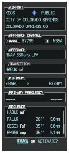
Figure 7-33 Barometric Minimums Set
