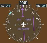
Figure 7-12 Assigned Heading of 290°
