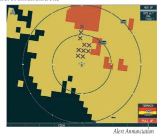
Figure 10-52 Alert Annunciation on the TAWS-B Page
