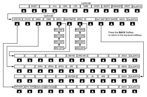
Figure 1-3 PFD Configuration Softkeys
