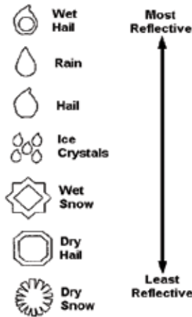
Figure 4-73 Precipitation Type and Reflectivity
