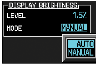
Figure 3-39 Aux Mode Display Brightness Mode Selection
