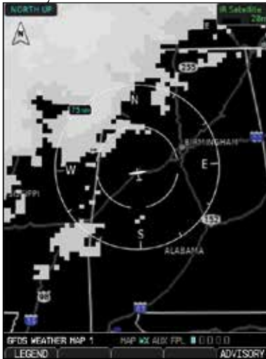
Figure 4-108 GCSS Infrared Satellite Data Map Display and Legend
