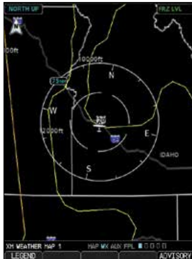
Figure 4-65 XM Weather - Freezing Levels
