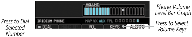
Figure 3-86 Select Soft Keys for Phone Volume Adjustment
