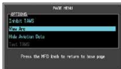
Figure 4-12 Select TAWS Display View (360 or Arc)
