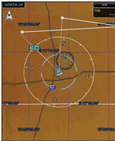
Figure 3-22 Navigation Map Field of View on the MFD
