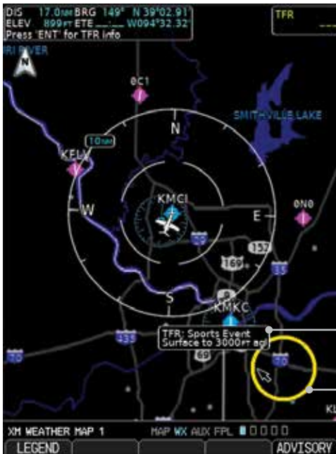
Figure 4-59 XM Weather - TFRs
