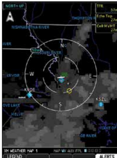
Figure 4-43 XM Weather - Echo Tops
