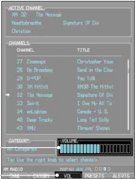
Figure 5-26 XM Radio Volume Setting
