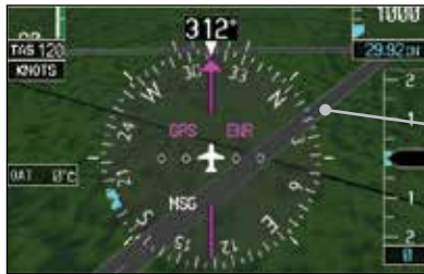
Figure 5-47 Depiction of Runway with a Loaded Flight plan
