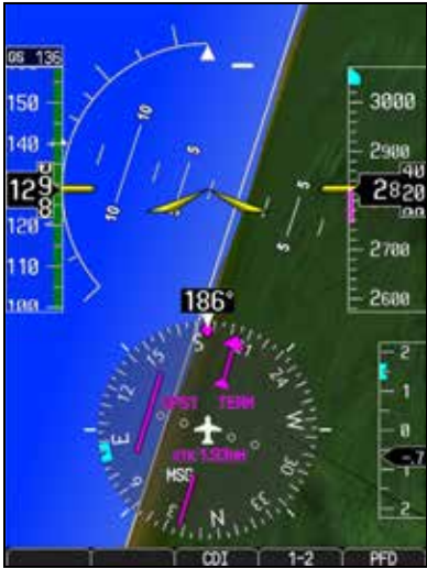
Figure 2-20 Extreme Roll Indication with Display Declutter
