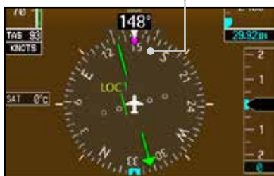
Figure 2-39 Auto-Slewing HSI with Localizer Backcourse Loaded (Shown with Corresponding Approach Plate)
