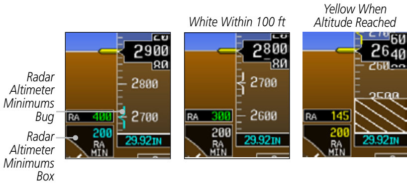
Figure 2-25 Radar Altimeter - Alerting Visual Annunciations
