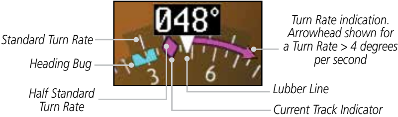
Figure 2-29 Turn Rate Indicator and Trend Vector
