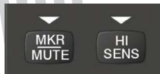
Figure 4-28 Marker Beacon Keys
