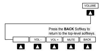
VOL -Decreases SiriusXM audio volume Increases SiriusXM audio volume VOI +**MUTE** Toggles SiriusXM audio on/off Returns to top-level softkeys BACK
