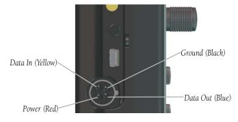
Power/Data Connector on the GPSMAP 695/696 Unit
