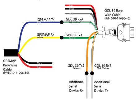
GPSMAP695/695 to GDL 39 Bare Wire Installation
