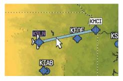
Flight Plan Page (Flight Plan Leg Highlighted with Map Pointer)
