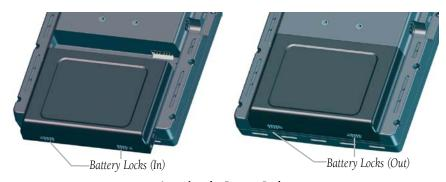
Inserting the Battery Pack
