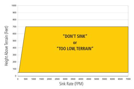
Figure 11-43 Negative Climb Rate (NCR) Sink Rate
