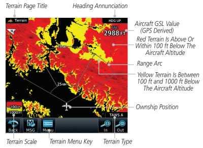
Figure 11-29 TAWS-A Page with Arc View
