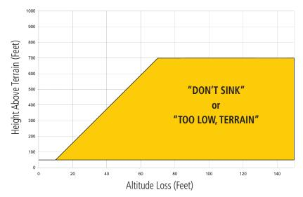
Figure 11-42 Negative Climb Rate (NCR) Altitude Loss
