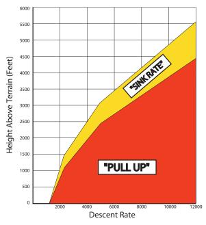
Figure 11-34 Excessive Descent Rate Alert Criteria
