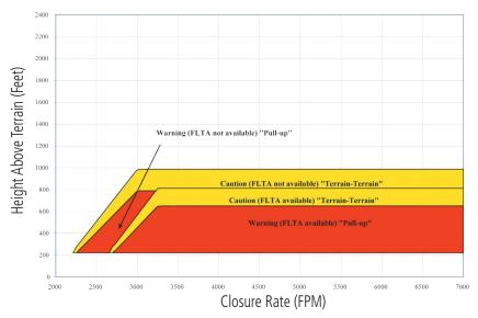
Figure 11-38 Excessive Closure Rate Alert Criteria (Flaps in Landing Configuration)
