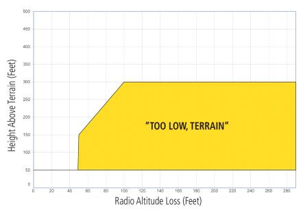
Figure 11-41 FIT Alerting After Takeoff
