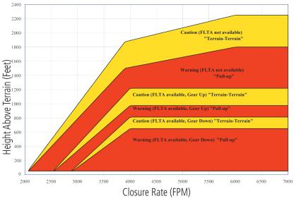
Figure 11-37 Excessive Closure Rate Alert Criteria (Flaps Up or Takeoff Configuration)
