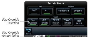
Figure 11-40 TAWS-A Page Menu and FIT Flap Override Annunciation
