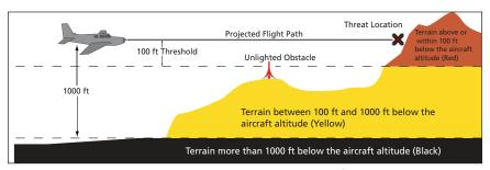
Figure 11-28 Terrain Altitude/Color Correlation for TAWS-A
