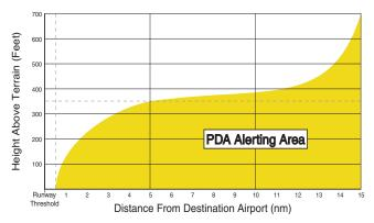
Figure 11-35 PDA Alerting Threshold
