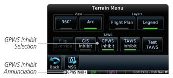
Figure 11-44 GPWS Inhibit Annunciation
