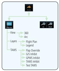
Figure 11-32 TAWS-A Page Functional Diagram
