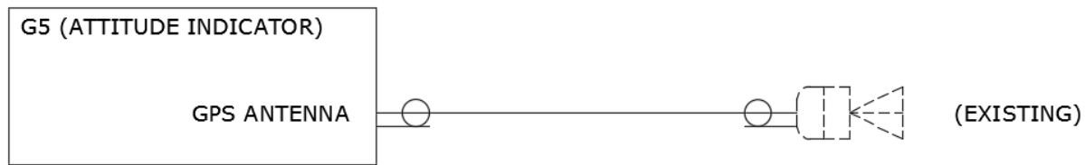
Figure 5-3 G5 (Attitude Indicator) with External GPS Antenna
