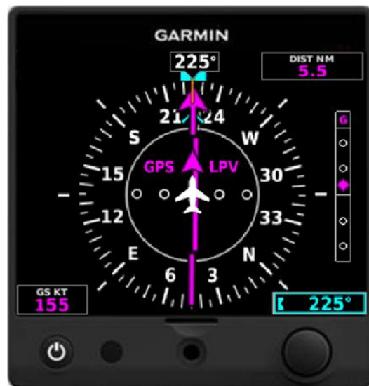
Figure 1-3 G5 Electronic Flight Instrument (DG/HSI)
