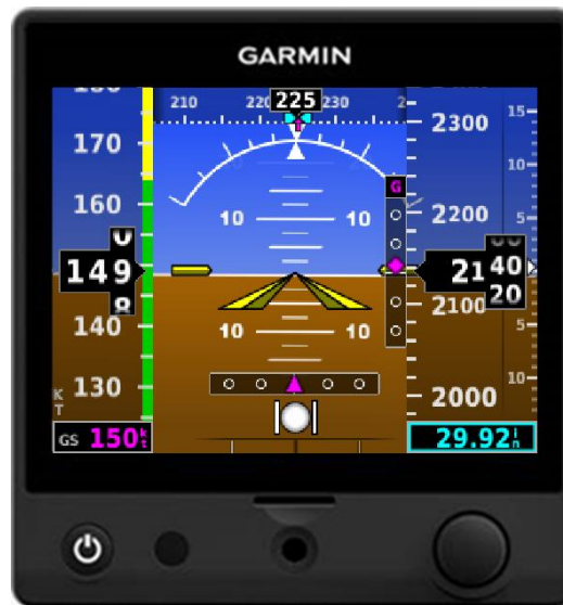
Figure 1-1, G5 Electronic Flight Instrument (Attitude)
