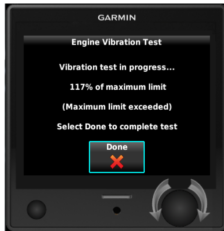
Figure 6-3 Engine Vibration Test Failure Indication
