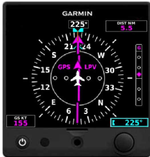
Figure 1-3 G5 Electronic Flight Instrument (DG/HSI)
