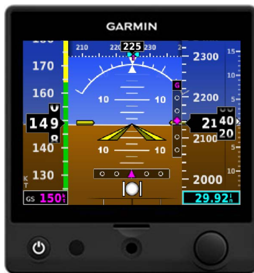
Figure 1-1, G5 Electronic Flight Instrument (Attitude)
