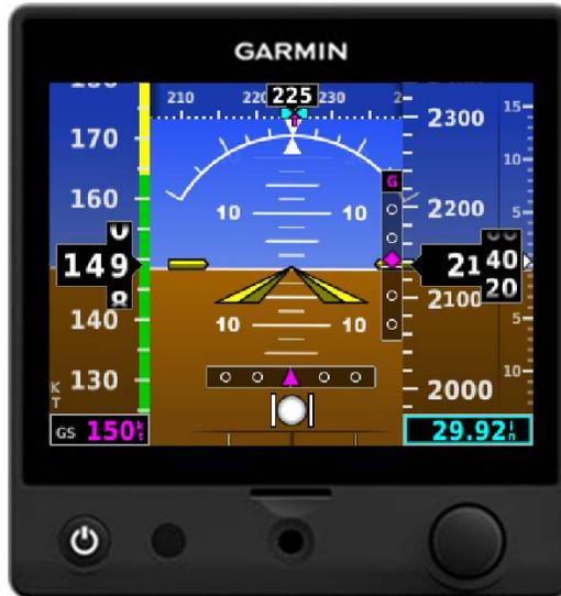
Figure 2-1 G5 Electronic Flight Instrument (Attitude)
