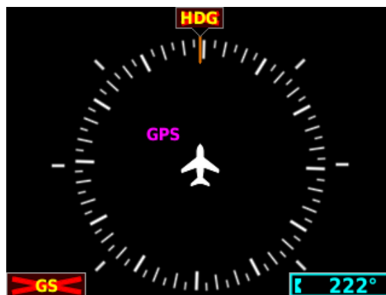
G5 HSI Failure Indications
