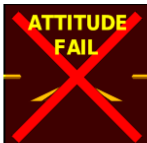
Attitude Failure Indication
