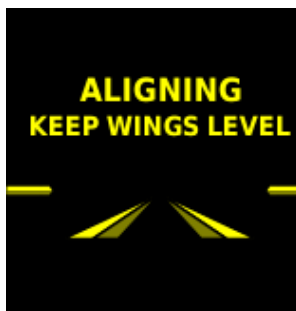
Attitude Aligned Keep Wings Level Indication
