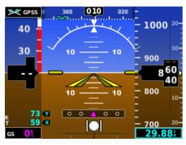
When GPSS is selected on the G5, GPSS turn commands are converted into a heading error signal to the autopilot. When the autopilot is operated in HDG mode, the autopilot will fly the turn commands from the GPS navigator. If
