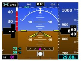
When GPSS is selected on the G5, GPSS turn commands are converted into a heading error signal to the autopilot. When the autopilot is operated in HDG mode, the autopilot will fly the turn commands from the GPS
