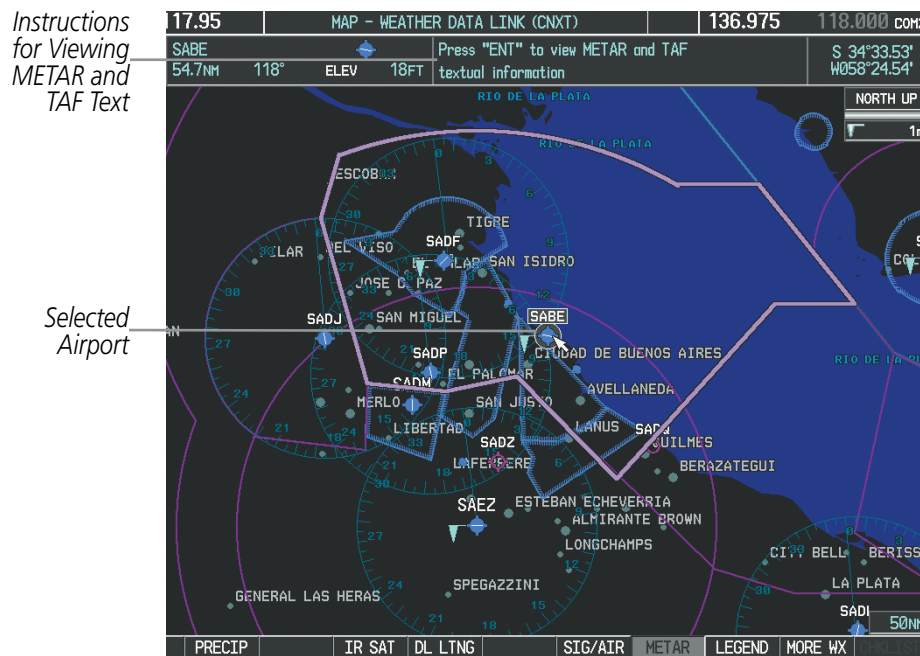
Figure 6-79 METAR Flags on the Weather Data Link (CNXT) Page
