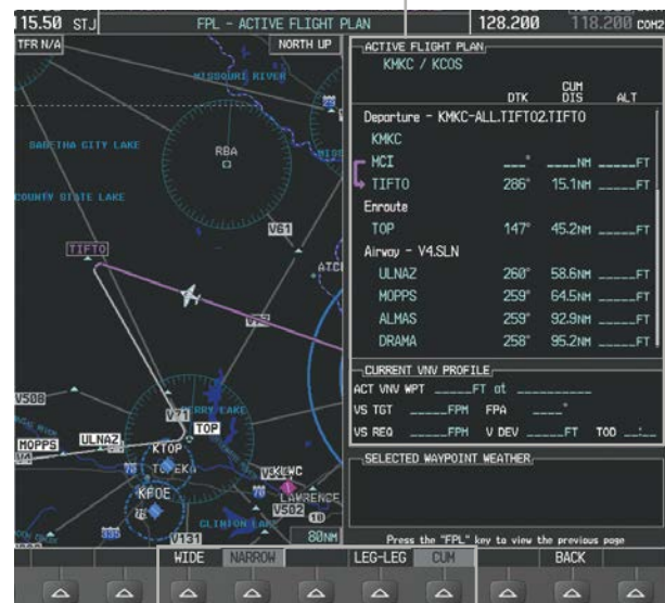
Active Flight Plan Cumulative Distance
