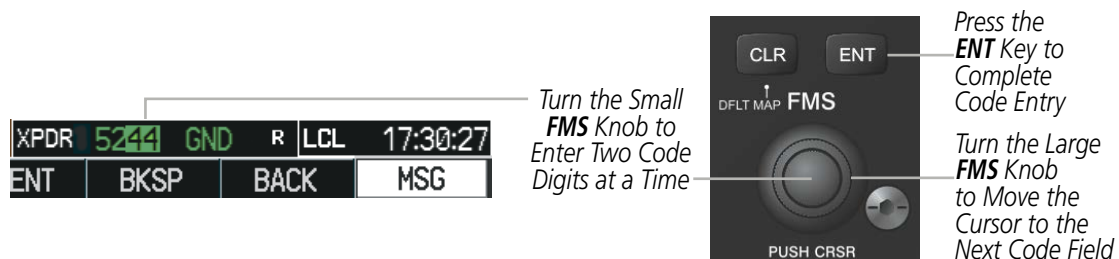
Figure 4-36 Entering a Code with the FMS Knob
