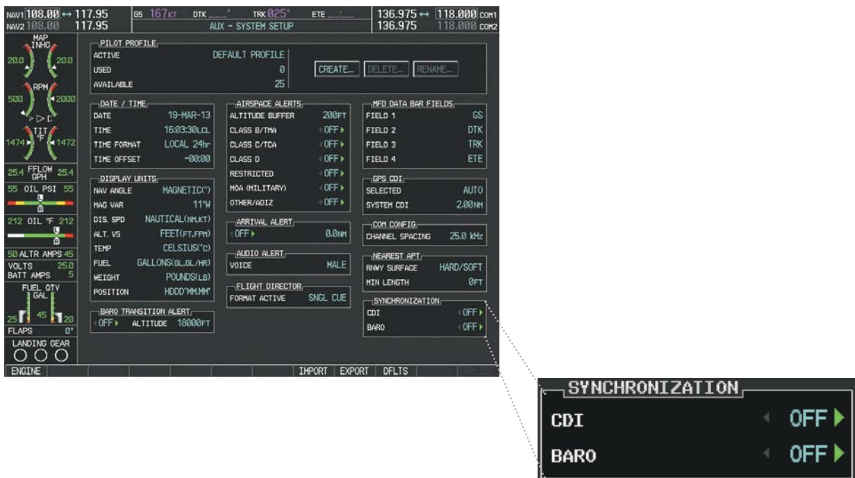
Figure 2-24 CDI Synchronization (AUX - System Setup Page)
