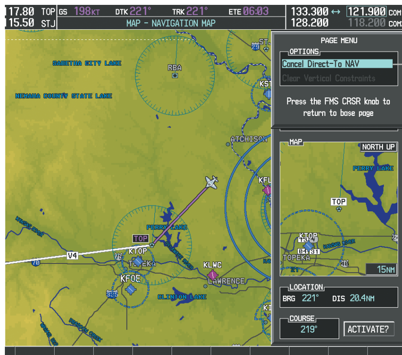
Figure 5-54 Direct-to Window - Cancelling Direct-to Navigation
