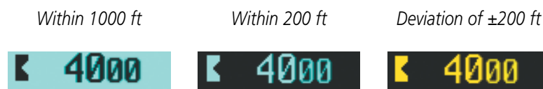
Figure 2-38 Altitude Alerting Visual Annunciations
