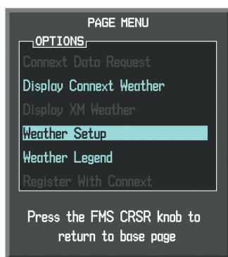
Figure 6-4 Weather Data Link (XM) Page Menu
