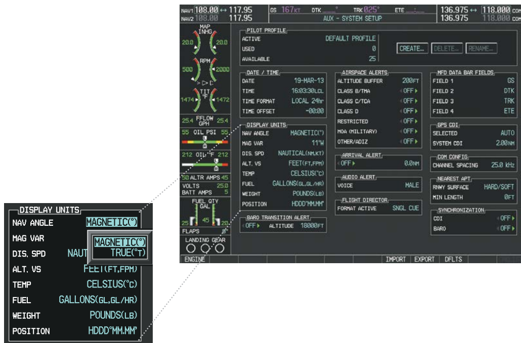
Figure 2-18 Navigation Angle Settings (AUX - System Setup Page)
