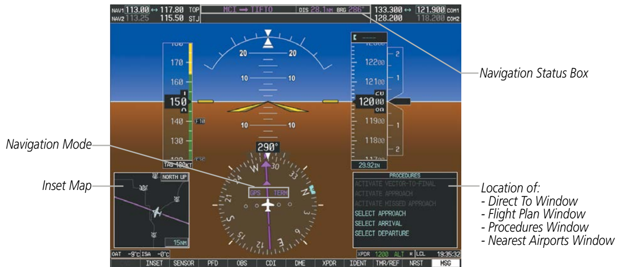
Figure 5-1 GPS Navigation Information on the PFD
