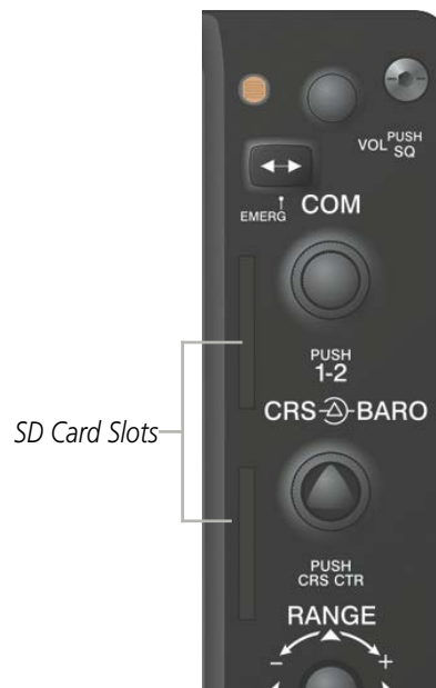
Figure 1-2 Display Bezel SD Card Slots
