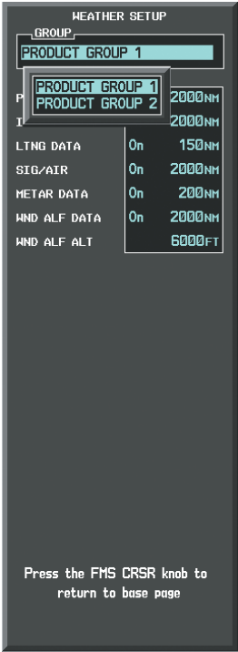
Figure 6-61 Weather Data Link (CNXT) Page Setup Menu
