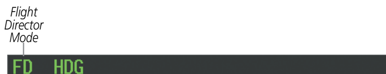
Figure 7-1 Flight Director Mode Engaged (G1000 AFCS Status Box)
