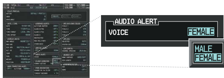
Figure A-6 System Setup Page, Alert Voice Settings
