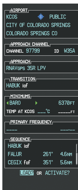
Figure 5-133 Barometric Minimums Set
