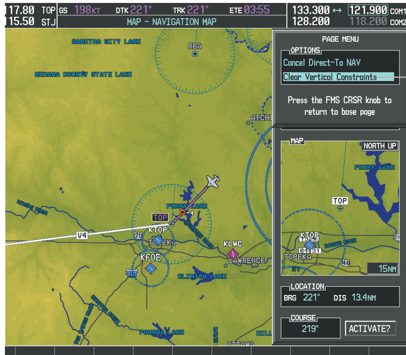
Figure 5-55 Direct-to Window - Clearing Vertical Constraints
