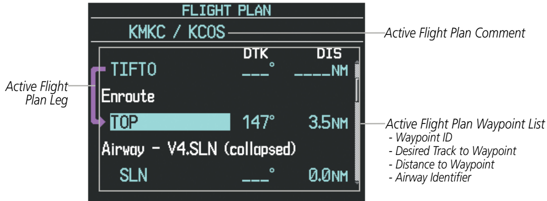
Figure 5-57 Active Flight Plan Window on PFD
