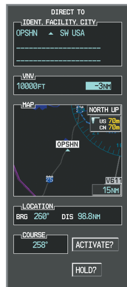
Figure 5-128 Enter VNV Offset Distance
