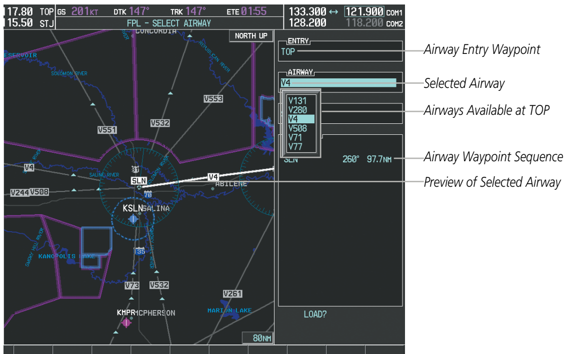
Figure 5-64 Select Airway Page - Selecting Airway
