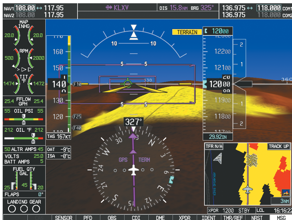
Figure 8-102 SVT Reversionary Mode
