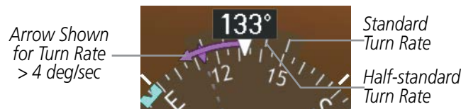
Figure 2-19 Turn Rate Indicator and Trend Vector
