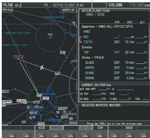
Active Flight Plan Leg to Leg Distance
