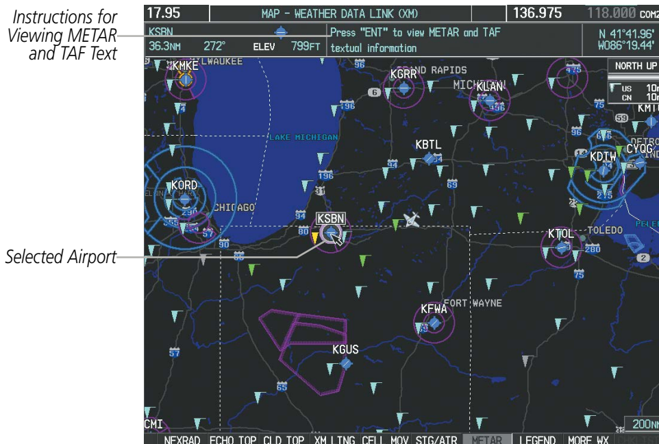
Figure 6-25 METAR Flags on the Weather Data Link Page
