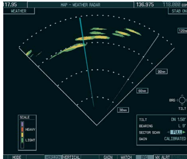
Figure 6-111 Selecting Sector Scan Position
