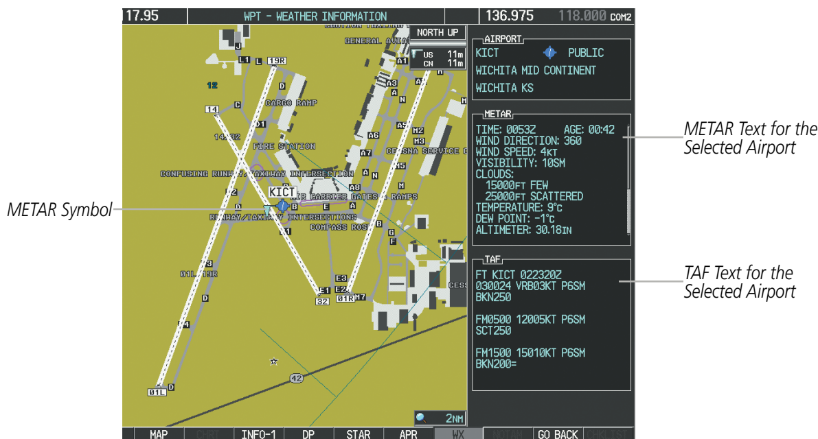
Figure 6-80 METAR and TAF Text on the Weather Information Page
