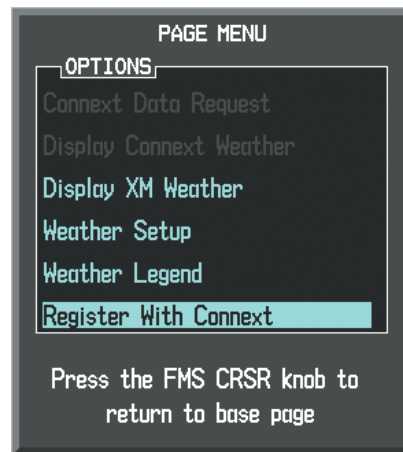
Figure 6-56 Select Register With Connex
