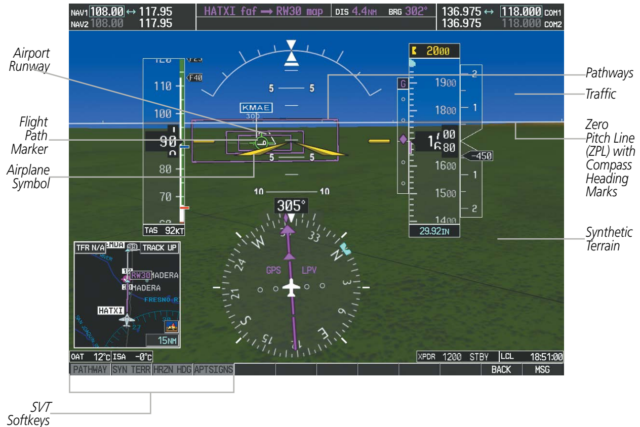
Figure 8-3 SVT on the Primary Flight Display
