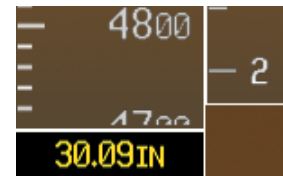
Barometric Settings not Synchronized on PFD displayed in yellow
