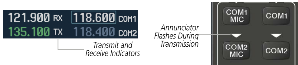
Figure 4-4 COM Radio Transmit and Receive Indications
