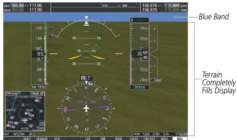
Figure 8-104 Blue Sky Bar with Full Display Terrain
