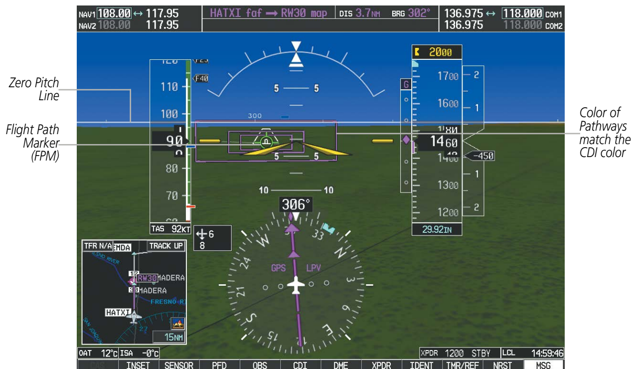
Figure 8-7 Flight Path Marker and Pathways
