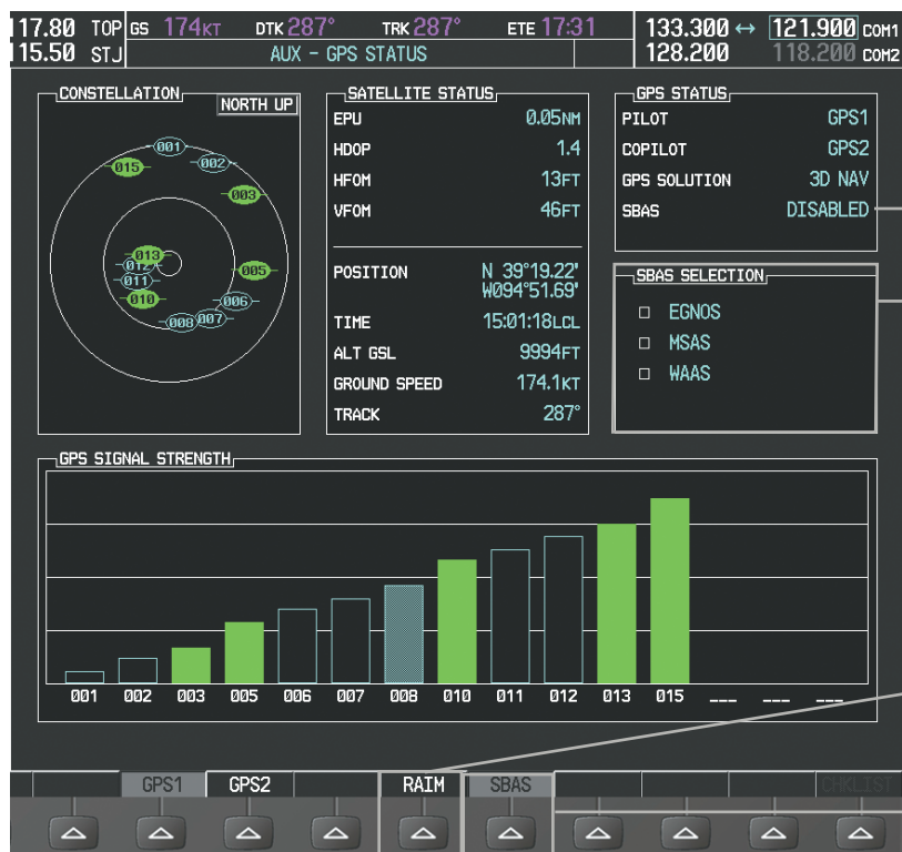
Figure 5-110 SBAS Display - Inactive
