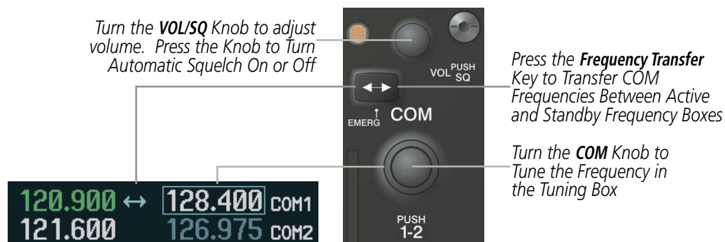
Figure 4-5 COM Frequency Tuning
