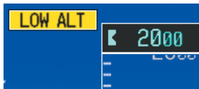
Figure 2-39 Low Altitude on GPS SBAS Approach
