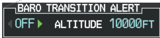
Figure 2-10 Baro Transition Alert (AUX - System Setup Page)
