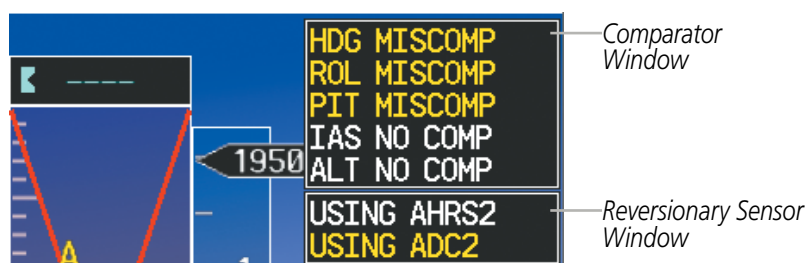
Figure A-3 Comparator and Reversionary Sensor Annunciation Windows
