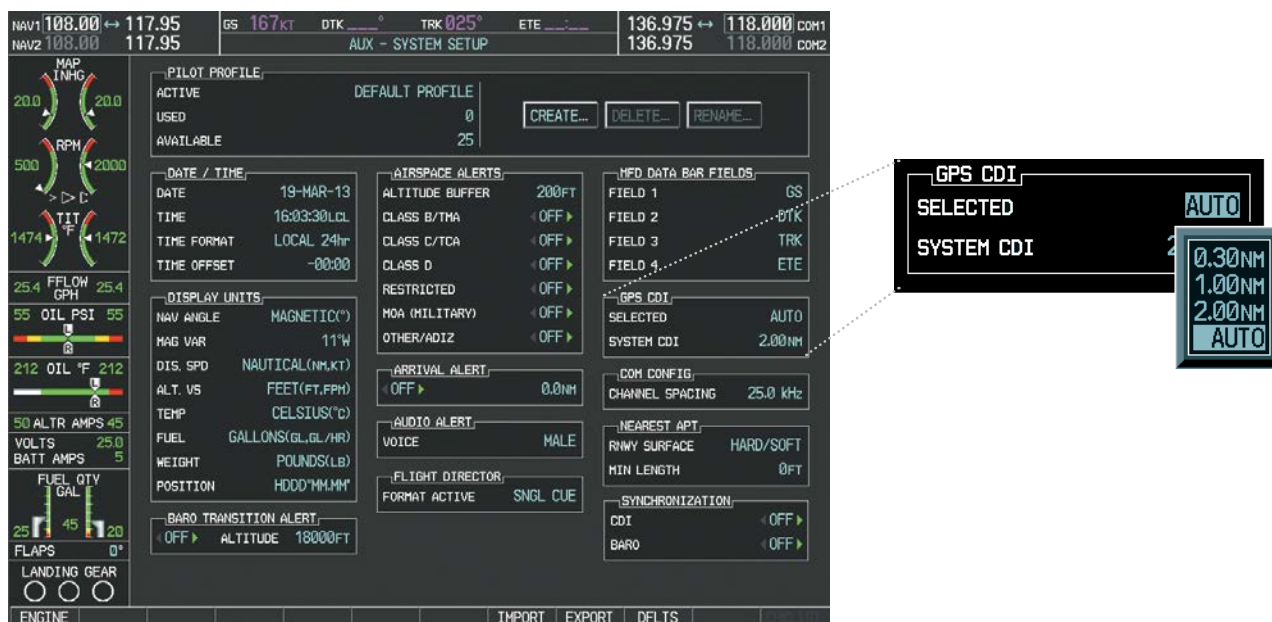
Figure 2-25 GPS CDI Setting (AUX - System Setup Page)
