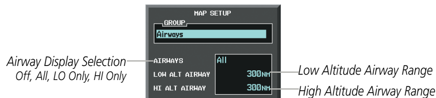
Figure 5-23 Navigation Map Setup Menu - AIRWAYS Setup
