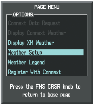
Figure 6-60 Weather Data Link (CNXT) Page Menu
