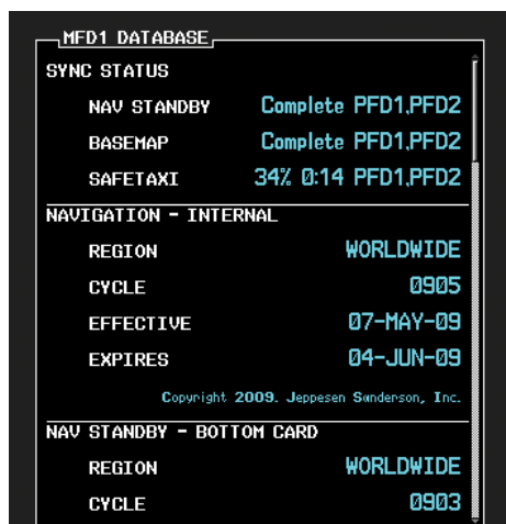
Figure B-8 AUX-System Status Page, Database Window
