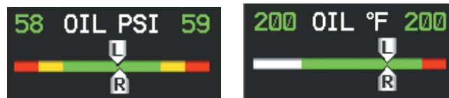
Figure 3-11 Oil Pressure and Temperature Gauges
