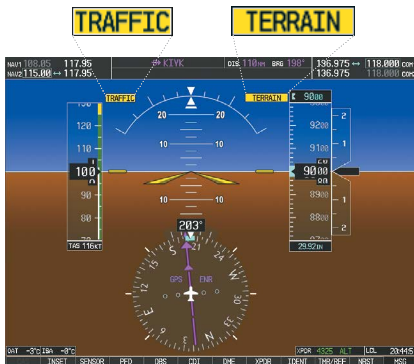
Figure 2-37 Traffic and Example TAWS Annunciations
