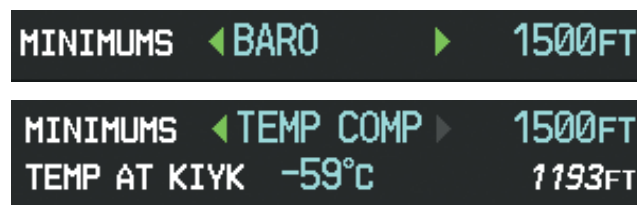
Figure 2-41 BARO and TEMP COMP MDA/DH
