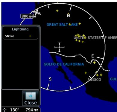
SXM displays a yellow cross icon to indicate a strike event occurring within a two kilometer region. Strike location is an estimate of its center. Unlike Stormscope, the icon does not change shape or color as data ages.
