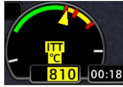
Timer displays once the parameter exceeds threshold. Automatic countdown begins.
