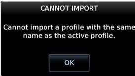
If imported profile has the same name as the active profile, overwrite option is not given. Acknowledge message, then activate a different profile and try again.
