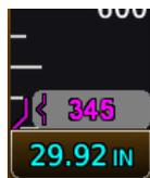
Compensating the approach minimums bug determines the location of the minimums reference on the altimeter. It does not adjust barometric altitude.
