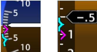
When receiving VNAV data from the navigator, a magenta chevron indicates the rate of descent needed to reach target altitude.
