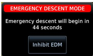
Once the 5 minute inhibit timer expires, the same pop-up warning appears regardless of whether EDM was triggered automatically or by the pilot.
