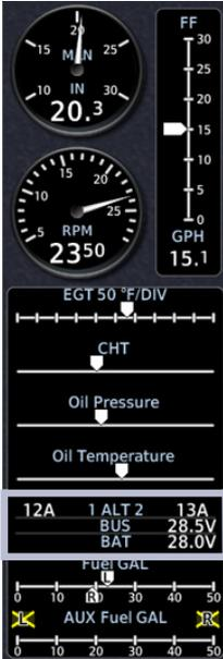
To accommodate more complex electrical systems, electrical gauges allow up to six parameters to display on three dedicated rows. These may include: • main generator • standby alternator • multiple buses • batteries
