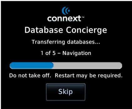
Database Concierge transfers databases from the app to Flight Stream 510. A progress bar shows when this process is complete.
