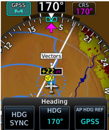
The **AP HDG REF** key is present if an autopilot is interfaced with the GDU and is configured to use GPSS emulation. This key changes the autopilot's heading reference between HDG bug and GPSS.
