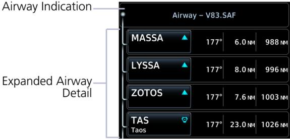
All airways begin with an indicator field and end with an exit identifier.
