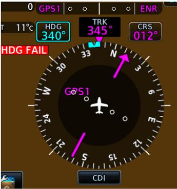
**HSI with Magnetometer Failure**
