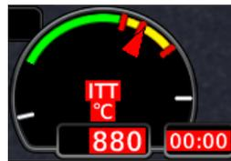
Timer changes color once it reaches zero. It flashes in unison with the alerted gauge pointer, value, and label, indicating a warning condition. Exceedance recording begins.
