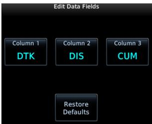
To select a flight plan data column, tap **Edit Data Fields**. Columns are arranged in numerical order (1 - 3).
