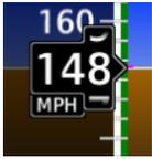
Airspeed indicator is configured at installation to meet the requirements of the AFM/POH. Available units: knots (default), kilometers per hour, and statute miles per hour.
