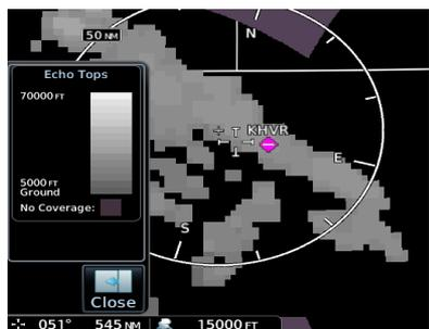
Depicts the location, elevation, and direction of NEXRAD radar echoes. This information is useful for gauging storm intensity in a relative sense. A higher radar echo means a stronger storm updraft.
