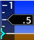
**Standard VSI:** This field replaces the trend indicator and moves up or down as the vertical speed changes. It displays only in expanded layouts.
