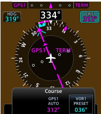
Selecting **VOR(1/2) PRESET** allows the pilot to preset VOR course selected course entries. Access this function by tapping the preset key and entering the value on the numeric keypad or by turning the inner control knob on the PFD.
