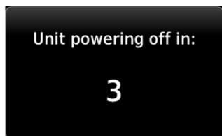
Pushing and holding the **Power** key for 4 seconds powers off the unit without safeguards. Shutdown occurs once the timer reaches zero.
