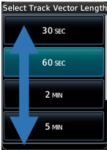
Scrollable lists group control keys related to a single function (e.g., selectable range options). When scrolling, all keys in the list are inactive.
