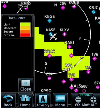
Turbulence is classified as light, moderate, severe or extreme. Turbulence data is intended to supplement AIRMETs and SIGMETs.
