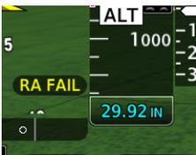
If the radar altimeter fails, the message "RA FAIL" annunciates in place of the current radar value.
