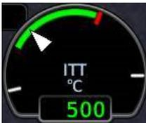
Once the system determines that the engine is running, the gauge changes to show the cruise red line limit.
