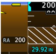
As the aircraft climbs, the ground band moves down the tape in equal amounts to the indicated RAD ALT value.
