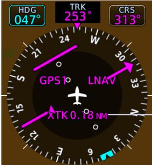
The GPS navigator determines CDI scaling. A cross track error displays if the CDI exceeds the full scale deviation value during GPS navigation.
