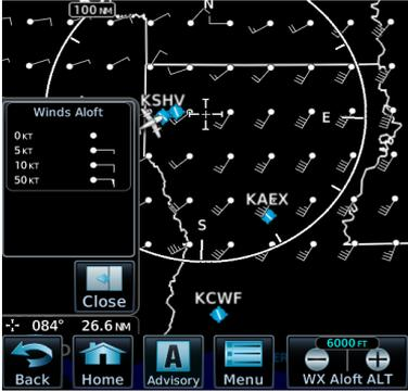
Indicates wind speed and direction for the specified altitude.
