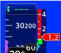
When the TCAS II LRU issues an RA, the VSI displays red no-fly bands to indicate areas to avoid. The green band indicates the desired climb/descent rate.
