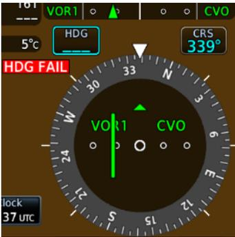
**HSI with GPS and Magnetometer Failures**
