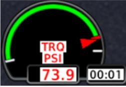
Exceedance timers indicate the maximum allowable time that the parameter can operate at an elevated level. This grace period is configured by the installer during initial setup. Depending on the parameter type, the time limit may be based on aircraft or engine manufacturer specifications.
