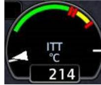
Once the system determines that the engine is starting, the gauge changes to show the starting temperature limits.
