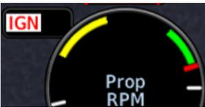
Text color and behavior (i.e., solid or flashing) are dependent upon configuration.
