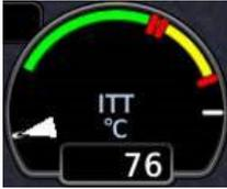
Configured by the installer to match the existing ITT gauge in the aircraft.
