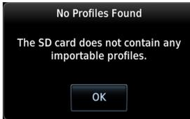
If SD card does not contain importable profiles, acknowledge message and replace SD card.
