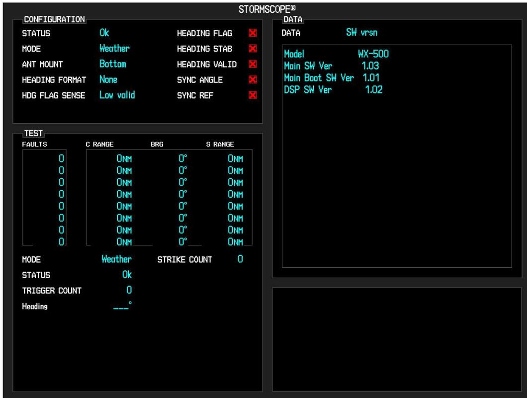
Figure 3-11, Stormscope Configuration Page
