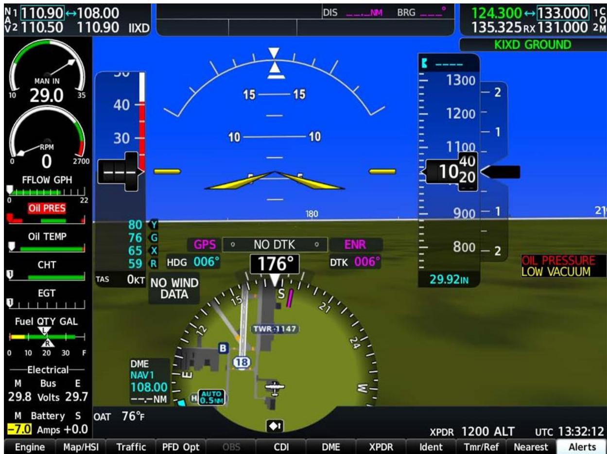
Figure 9-4, GDU Reversionary Mode
