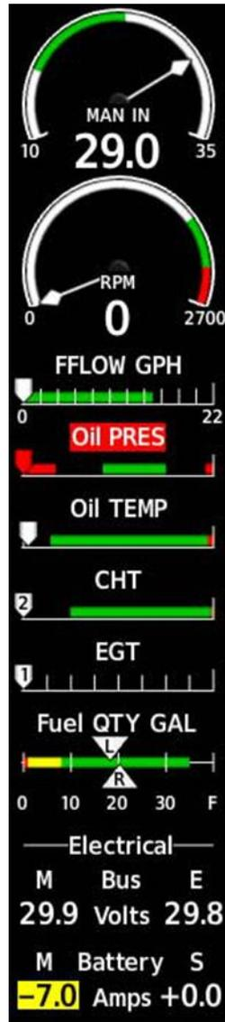
**Figure 7-3, Normal Engine Instrument Markings (MFD)**
