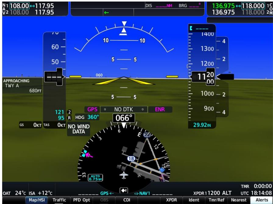
**Figure 7-7, Normal Mode AHRS Check**
