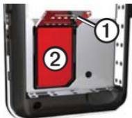
2. Place the SIM card ② in the device with the gold contacts facing down and the notched corner near the bottom of the device.
