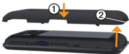
2. Locate the battery cover notch ② on the bottom of the device.
