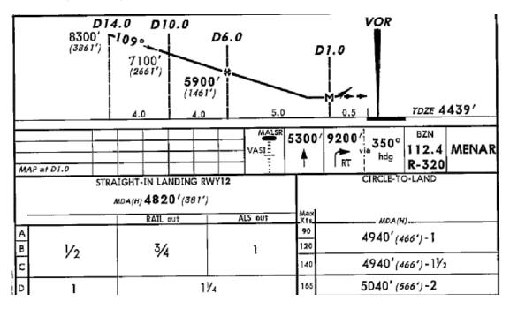
This approach is the GPS 12 approach to KBZN and has a couple of interesting twists to it. The profile view of the GPS 12 approach shows a vertical path with a solid black line, but no mention of an Lnav/Vnav minimum. In this case, the MAP is offset from the end of the runway by a half mile. This waypoint MADSE, is the D1.0 fix shown above and is the MAP which is the point the vertical path will be built from.
