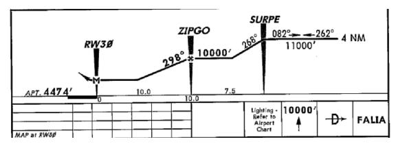
Shown above is an excerpt from the RNAV GPS-A circling approach to KBZN. This approach is an Lnav only approach and does not support vertical guidance, since the RW30 waypoint does not have an altitude and vertical path associated with it. The VDI will remain flagged throughout the approach. If this approach depicted a light grey dashed line vertical profile at ZIPGO, then the GNS 480 would support vertical guidance.
