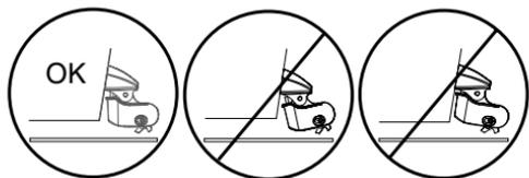
Adjust the speed sensor so it is parallel with the bottom of the boat. If the speed sensor is not adjusted properly, the sonar may experience inaccurate or degraded speed readings.
