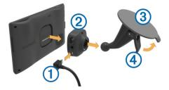
2 Press the mount ② onto the suction cup ③ until it snaps into place.
