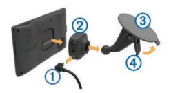
2 Press the mount ② onto the suction cup ③ until it snaps into place.
