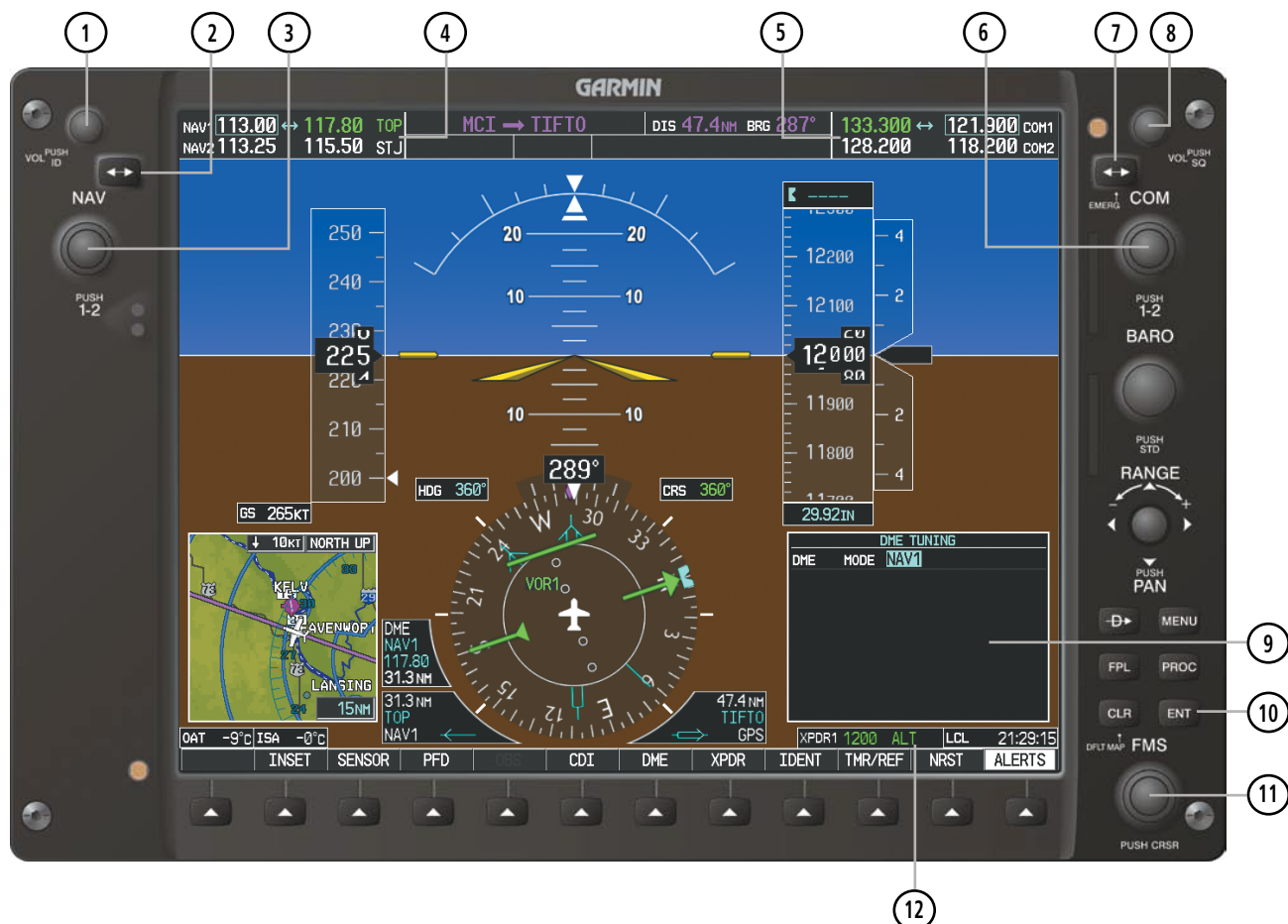
Figure 4-1 PFD Controls, COM/NAV Frequency Tuning Boxes, and DME Tuning Window
