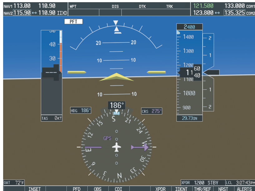
Figure 6-9. GFC 700 Pre-Flight Test
