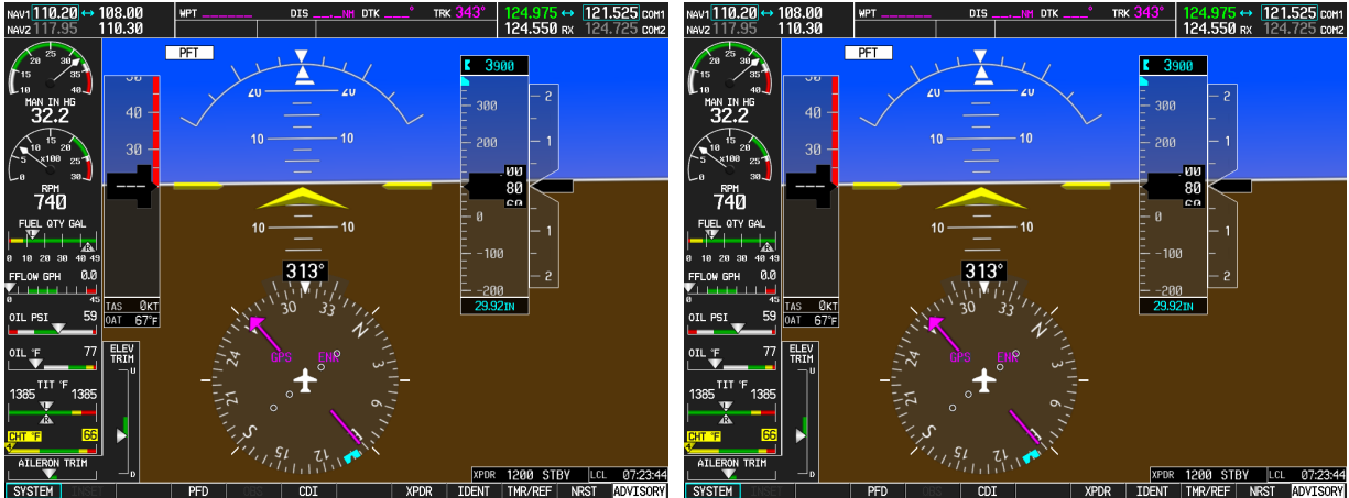
Figure 6-2. G1000 Reversionary Mode Check
