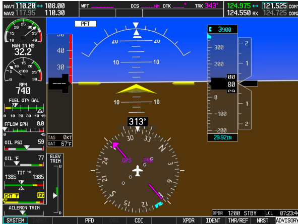
Figure 3-7. MFD Failure Mode
