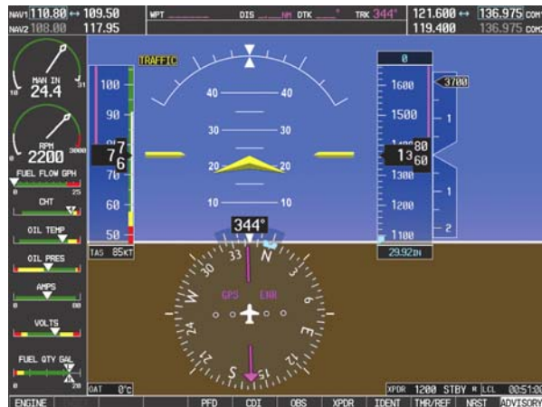
Figure 3-6. MFD Failure Mode
