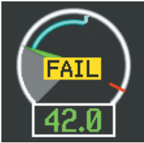
Engine Failure Indication
