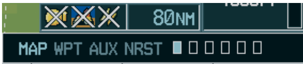
Loss of Hazard Functions with Loss of GPS Position
