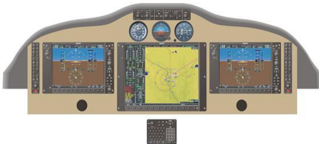
Figure 2-5. Three Display Installation
