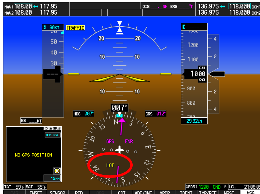
Figure 7-3. Loss Of Integrity Annunciation
