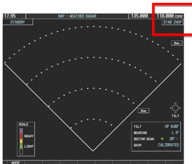
Figure 5-37. Weather Radar Page (STAB INOP)
