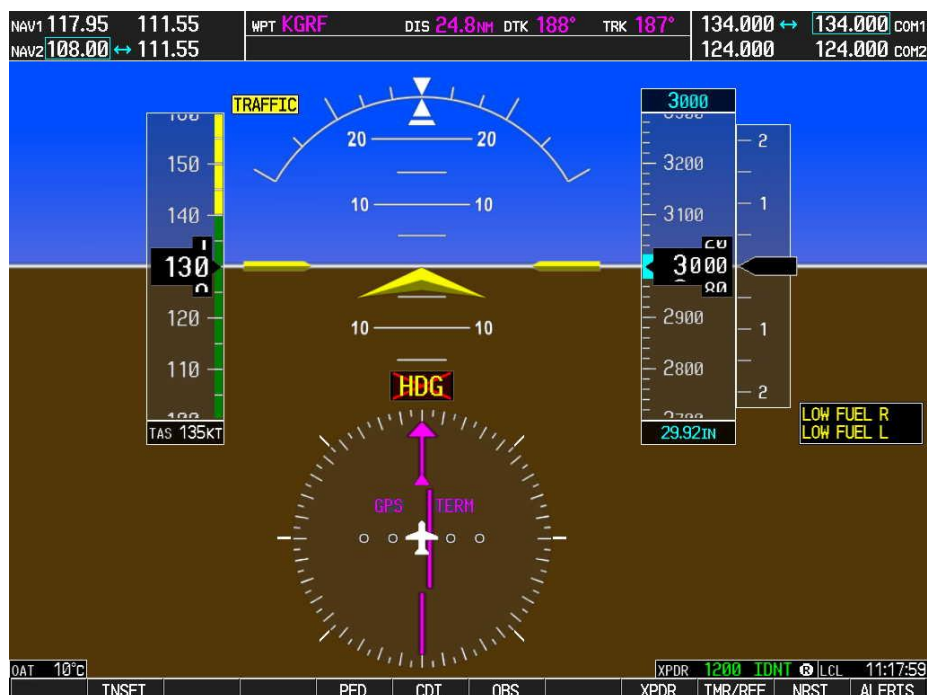
Figure 5-14. Heading Failure Indication
