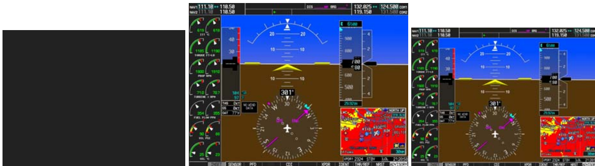
Figure 2.2 – Reversion with PFD1 failure
