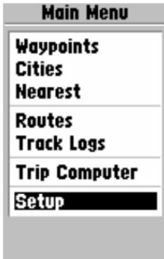
The Main Menu Page on the GPS III/III+/12Map/Navtalk. Select 'Setup' to make the desired interface settings.
