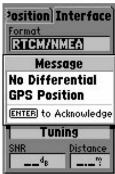
If the 'No Differential GPS Position' message is displayed on your GPS receiver, correction data may not be available. This may be due to a missing or weak beacon signal, not enough GPS satellites or bad wiring connection between the GBR 21 and GPS.
