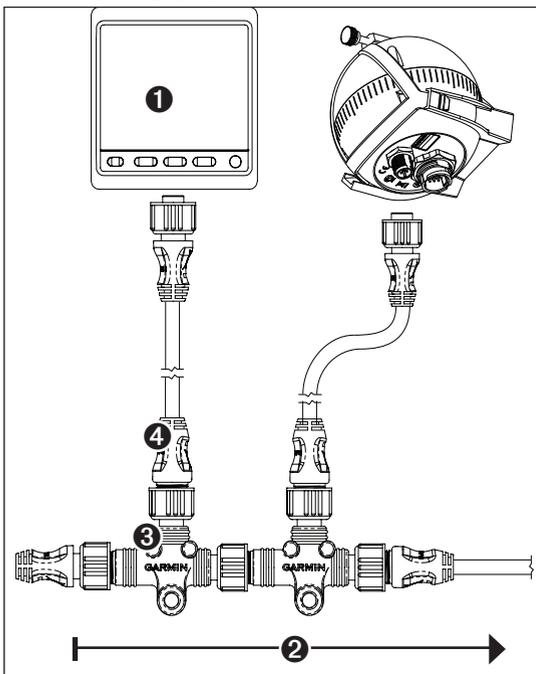
2. Disconnect one side of a NMEA 2000 T-connector from the network.
