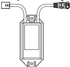
The Autopilot Gateway allows the GHP 10V autopilot system to steer the boat through the Volvo™ steering system. The Autopilot Gateway connects to the CCU through the CCU interconnect cable and connects to the Volvo steering system using a proprietary Volvo connector.
