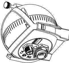
The CCU acts as the brain of the GHP 10V. The CCU contains the sensory equipment used to determine heading. The CCU connects to the Autopilot Gateway with a single cable. The CCU also connects to a NMEA 2000® network to communicate with the GHC 20, and to optional NMEA 2000-compatible GPS devices ([page 9](#)).
