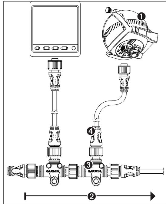
2. Disconnect one side of a NMEA 2000 T-connector from the network.
