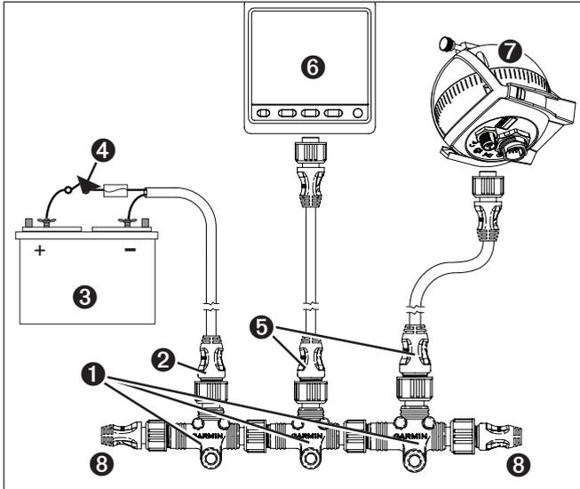
2. Connect included NMEA 2000 power cable ❷ to a 12 Vdc power source ❸ through a switch. Connect to the ignition switch ❹ of the boat if possible, or through an in-line switch (not included).
