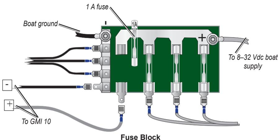
**CAUTION:** The GMI 10 maximum input voltage is 32 Vdc. Do not exceed this voltage, because this can damage the GMI 10 and void the warranty.
