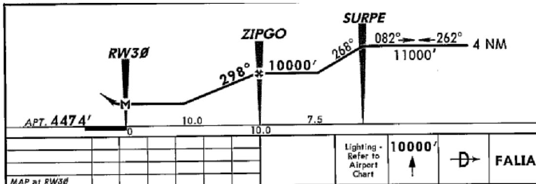
Shown above is an excerpt from the RNAV GPS-A circling approach to KBZN. This approach is an Lnav only approach and does not support vertical guidance, since the RW30 waypoint does not have an altitude and vertical path associated with it. The VDI will remain flagged throughout the approach. If this approach depicted a light grey dashed line vertical profile at ZIPGO, then the GNS 480 would support vertical guidance.
