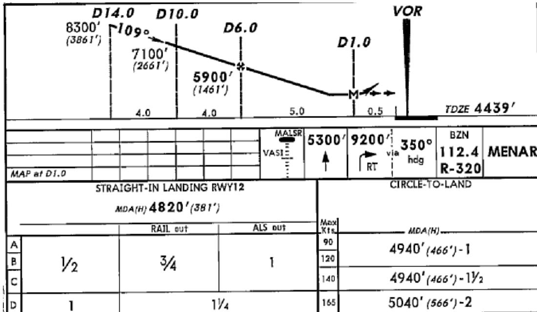
This approach is the GPS 12 approach to KBZN and has a couple of interesting twists to it. The profile view of the GPS 12 approach shows a vertical path with a solid black line, but no mention of an Lnav/Vnav minimum. In this case, the MAP is offset from the end of the runway by a half mile. This waypoint MADSE, is the D1.0 fix shown above and is the MAP which is the point the vertical path will be built from.
