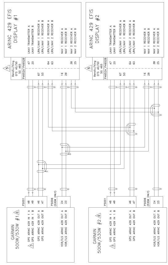
Figure H-10. ARINC 429 EFIS Interconnect Sheet 1 of 2
