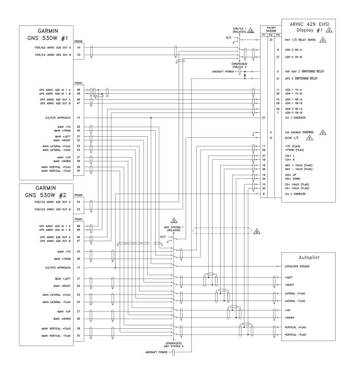
Figure H-12. ARINC 429 Sandel EHSI Interconnect (Two GNS 530W, One Sandel SN3308) Sheet 1 of 2
