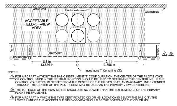
Figure 2-2. Source Selection Annunciation Field of View
