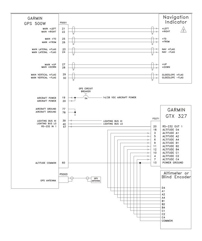
Figure H-3. GPS 500W Typical Installation Sheet 1 of 2
