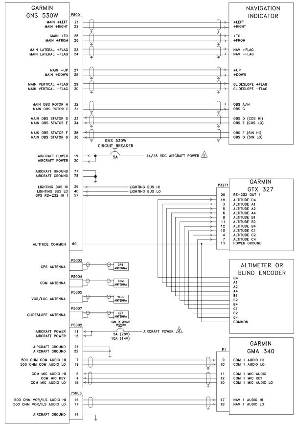
Figure H-2. GNS 530W Typical Installation Sheet 1 of 2
