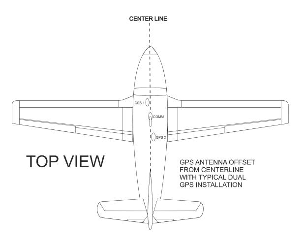
Figure 2-1. GPS Antenna Installation Considerations
