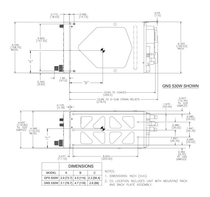
Figure F-1. GNS 530W Mounting Rack Dimensions
