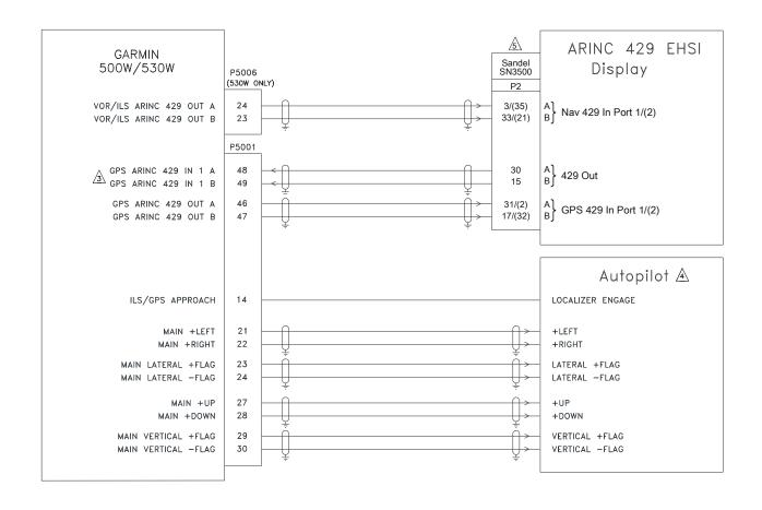
Figure H-28. ARINC 429 Sandel EHSI Interconnect (One 500W Series Unit, One Sandel SN3500) Sheet 1 of 2
