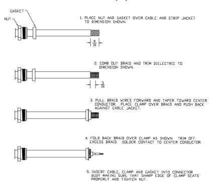
Figure 3-1. Coaxial Cable Installation
