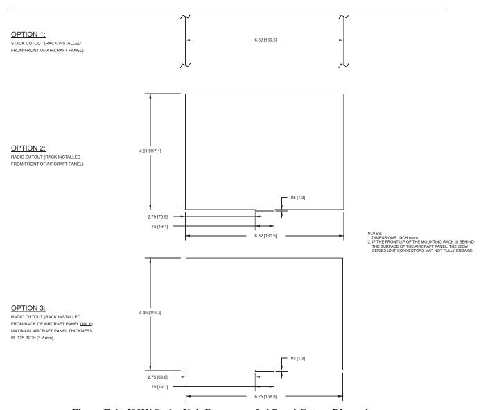
Figure F-4. 500W Series Unit Recommended Panel Cutout Dimensions
