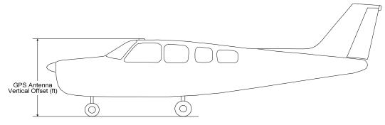
Figure 5-17. Measurement of GPS Vertical Offset
