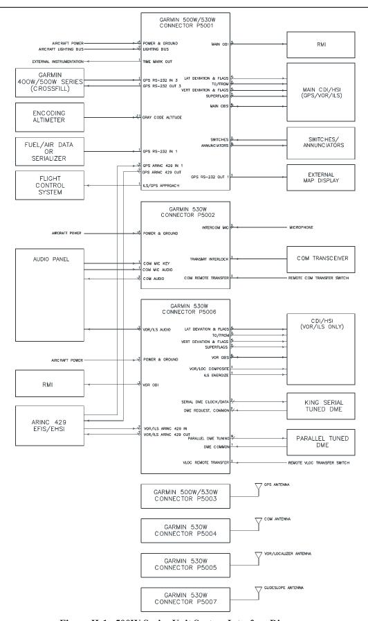
Figure H-1. 500W Series Unit System Interface Diagram
