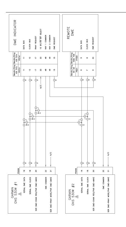
Figure H-22. King Serial Remote DME Tuning Interconnect
