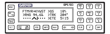
The front panel consists of a 3- line, 22- character LCD display and 21 keys. Both the display and keypad are illuminated for your convenience while operating in the darkness.
