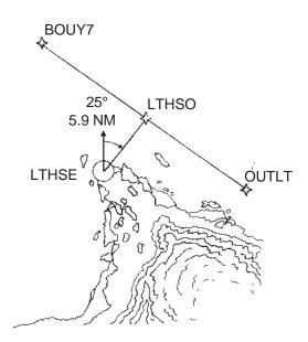
Suppose you are navigating around the coastline of a point with a lighthouse as illustrated above. You need to know when you pass abeam the lighthouse so that you can turn inland but, due to poor visibility, you cannot see the lighthouse. The CPA function will help you find your way!
