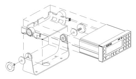
The GPS 100 comes with a standard slide-in gimbal bracket for fixed installations. The gimbal bracket may be mounted on a flat surface or overhead using screws or bolts.
