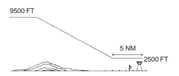
Suppose you are travelling from Denver, Colorado to the Beech factory in Wichita, Kansas. You are flying VFR at 9,500 feet MSL. You wish to be at 2500 feet (500 feet above Beech's traffic pattern altitude) 5 nautical miles from the airport. Additionally, you wish to descend at 1000 feet per minute. Enter the above data on the VNAV Planning page and turn the VNAV function on.
