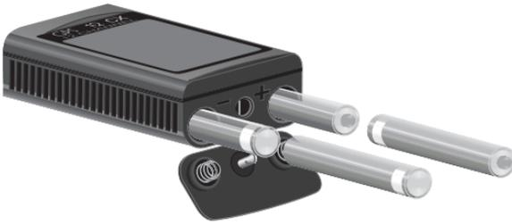
The GPS 12CX operates on 4 AA batteries (included), which are installed at the base of the unit. These batteries provide up to 36 hours of use in “Power Saver” mode.
