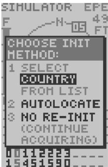
To access the EZ-Init feature, without satellite coverage press **ENTER** while the Satellite Status Page is displayed.
