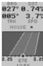
*This example indicates that you are off course to the left and need to steer right to get back on course. Continue turning in the direction of the highway until the highway is pointing straight up, then continue in that direction.*
