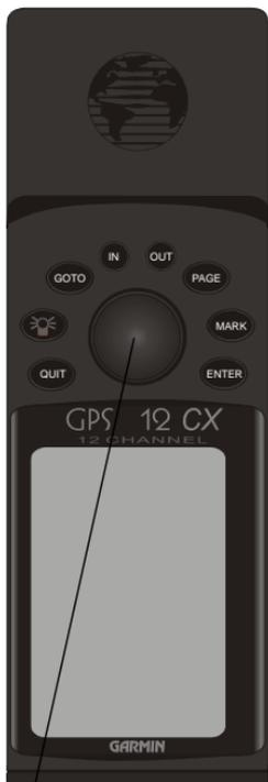
Press the **ROCKER** key up or down to select letters or numbers in a data field. Pressing the **ROCKER** key left or right, moves the cursor forward or backward along the data path.
