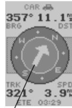
The **POINTER** indicates the bearing (BRG) to the destination waypoint. When navigating, turn in the direction of the pointer until the pointer is straight up, then continue in that direction. A quick check to verify that you are indeed traveling in the right direction, if the bearing and track are the same then you are exactly on course.
