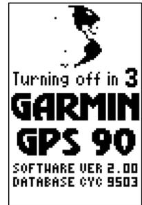
*The power off count-down helps prevent the GPS 90 from being powered down accidentally.*
