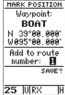
If you're heading out without a planned route, the mark function can be used to quickly create a route back to your starting point.
