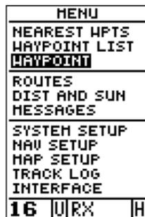
Use the arrow keypad to select a submenu from the menu page. Press **ENTER** to access the selected submenu.
