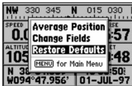
'Restore Defaults' will override any data field changes you've made to the Position Page, reverting back to the factory default settings.
