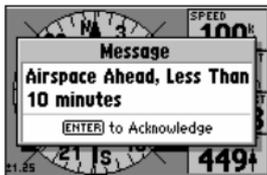
When you are projected to enter an airspace, the first alert is typically 'Airspace Ahead Less Than 10 minutes'.
