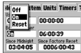
The battery timer will automatically reset when depleted batteries are replaced with a fresh set.
