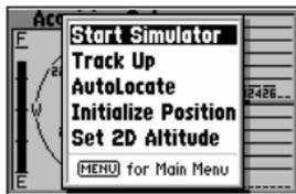
The Satellite Status Page Options allow you to enable the built-in simulator, change the sky view orientation or initialize the receiver.
