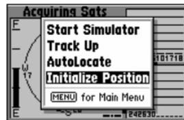
*'Initialize Position' is used to designate your approximate position directly on the map display. The receiver uses this information to determine which satellites should be in view.*
