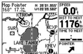
User waypoints can be created directly from the Map Page, by placing the panning pointer on the desired position and pressing ENTER.
