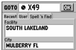
By placing the panning pointer over an on-screen waypoint and pressing GOTO/ NRST, you won't have to manually enter the identifier for the waypoint.
