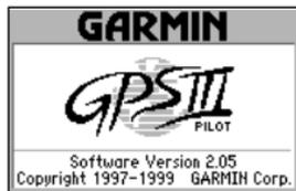
*The Welcome Page is displayed when the GPS III Pilot is first turned on. During this time the receiver is conducting a self-test.*
