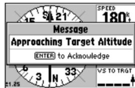
*Once you are within 500 feet of the target altitude, the 'Approaching Target Altitude' message will appear and the VNAV indicator will be removed from the HSI display.*
