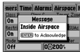
*Due to vertical airspace limits, if you fly above or below an airspace then descend or climb into the airspace, the 'Inside Airspace' message may be the only alert provided.*
