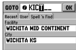
Press ENTER and use the rocker keypad to enter the identifier of the destination waypoint. Press ENTER to begin navigation.
