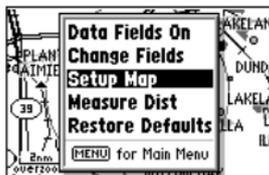
'Setup Map' allows you to change map orientation, background map detail, on-screen Jeppesen data, text size, etc.
