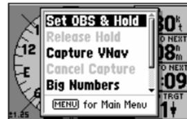
The 'Set OBS and Hold' option allows you to specify an inbound heading to a destination waypoint.
