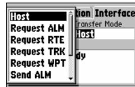
When transferring data to/from another unit, select the type of data and whether to 'request' it from or 'send' it to the other unit.
