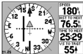
This example shows the aircraft heading parallel to the desired course, with the aircraft right of course more than 0.5 nm.
