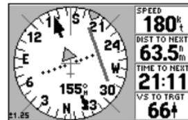
Use the rocker keypad to select the desired OBS heading. Note the heading at bottom center of HSI display (155° in this example).
