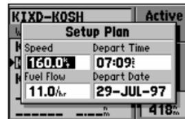
'Setup Plan' allows you to define planned speed, fuel flow and departure time in order to review trip planning figures.
