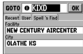
To GOTO a waypoint, press GOTO/NRST and highlight the waypoint identifier field at the top of the page.
