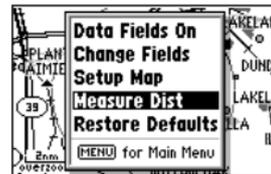
*When using the 'Measure Dist' option, an arrow appears with an 'Enter Reference' prompt. Point to the initial reference point and press ENTER.*
