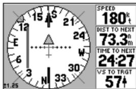
When off course beyond the limits of the CDI scale, the D-bar will appear in gray and stay at the edge of the scale (until your off course error is less than the limits of the scale).
