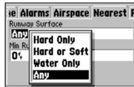
*'Hard Only' includes only concrete, asphalt, or similar sealed surface runways.*
