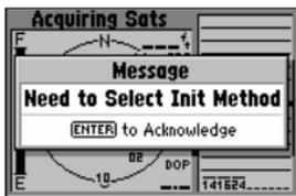
*When new (or if a position cannot be determined after 10 minutes), the GPS III Pilot will prompt you to initialize the receiver. The unit needs a starting position to determine which satellites are in view.*
