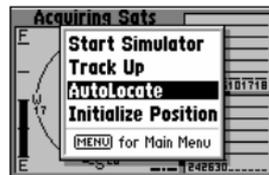
*'AutoLocate' forces the receiver to search for all satellites (twelve at a time) until enough satellites are found to determine a position.*
