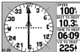
From the HSI Page, you can increase/decrease the simulated speed using the UP/DOWN keys on the rocker keypad.
