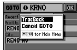
*'TracBack' allows you to retrace your path based upon an automatic track log recording.*
