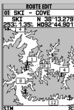
The GPSMAP 175's route edit mode also allows you to insert a new route waypoint in any route leg using the map cursor.
