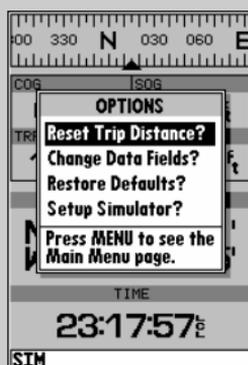
The GPSMAP 175's position page features a context-sensitive options page that provides access to functions and features relating to the position page.
