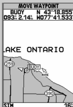
The GPSMAP 175's main menu page features four waypoint submenus that let you manage a large number of waypoints quickly and efficiently. The submenus also provide a continuously updated nearest waypoints list and a proximity waypoint alarm function that can be used to define an alarm circle around submerged hazards, shallow waters, etc.
